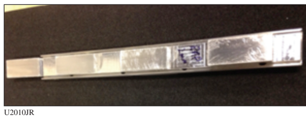
Figure 144.113 Photograph showing the specifically designed multichannel crystal for the XRS Rowland spectrometer on OMEGA.
