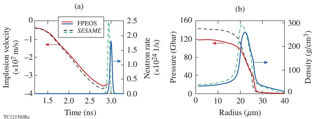
The figure compares the implosion prediction between *SESAME* EOS (dashed line) and FPEOS (solid line) of CH: (a) the implosion velocity and neutron-production rate as functions of time and (b) the pressure and density as functions of target radius at peak neutron production.
