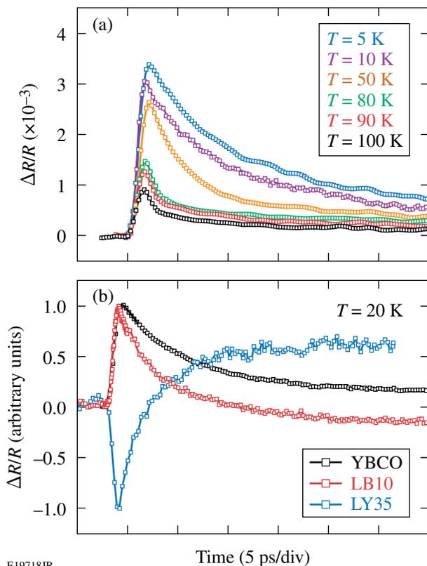
Figure 127.26 (a) The photoresponse  $\Delta R/R$  transient versus delay time for a 100-nm-thick YBCO film at different temperatures. (b) The normalized  $\Delta R/R$  waveforms versus delay time measured at 20 K for the reference YBCO film and the LY10 and LY35 S/F bilayers.
