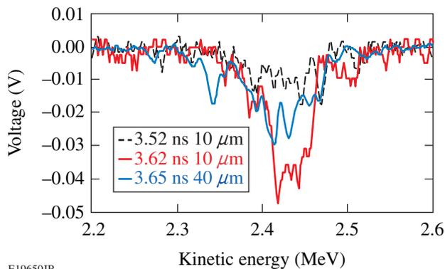
Figure 125.18 Time-of-flight spectra of 2.45-MeV neutrons from thermonuclear  $\text{d}(\text{d},\text{n})^3\text{He}$  reactions in integrated fast-ignition experiments. Spectra with various timings of the OMEGA EP beam are shown for two target types.
