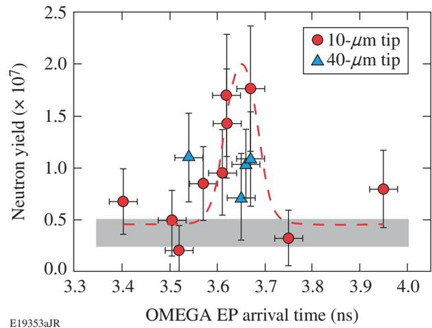
Figure 125.19 Measured neutron yield as a function of the arrival time of the short-pulse laser for two types of cone targets: 10- $\mu\text{m}$  (circles) and 40- $\mu\text{m}$  (triangles) tip diameter. The gray area represents data without the short-pulse laser.
