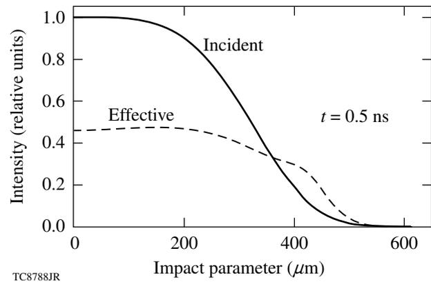
Figure 122.15 Incident (super-Gaussian with an index  $n = 4$ ) and effective beam profiles at  $t = 0.5$  ns for the same simulation with nonlocal transport and CBET as shown in Fig. 122.14. The effective profile emulates the loss ( $\approx 26\%$ ) and redistribution of the energy inside the beam caused by CBET.
