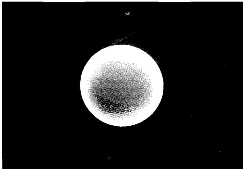
Fig. 32 Fusion target fuel core-mounted using two silk fibers in the geometry of a colliding shell target.
