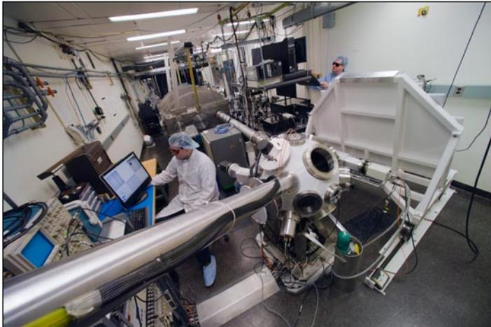
Shown is a broader view of the MTW target area where Philip Nilson is aligning the target as viewed on a computer monitor, while Michael Storm is preparing an on-shot laser-temporal diagnostic. A long collimation tube attached to the MTW target chamber supports a charge-coupled-device (CCD) camera (not visible) operating as an x-ray spectrometer in the single-photon-counting mode. Movable lead shielding protects an adjacent area from high-energy x rays produced during some target shots.
