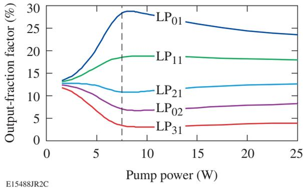
Figure 110.54 Output-fraction factors of LP fiber modes versus pump power from the localized model. The dashed vertical line is the pump threshold for saturation.
