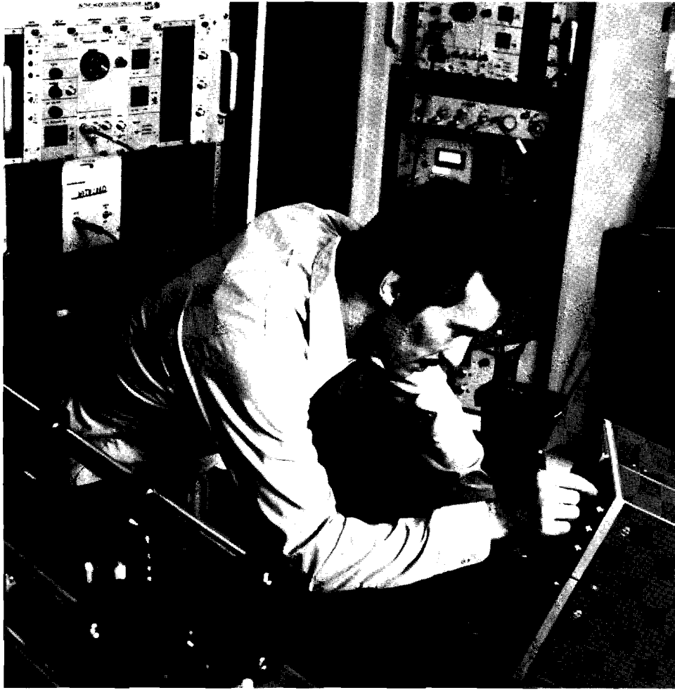
Georg Albrecht, LLE staff scientist, is preparing for fine adjustment of a Kuizenga oscillator, part of which is visible in the lower left. In the background are the electronic controls for two of these oscillators.
