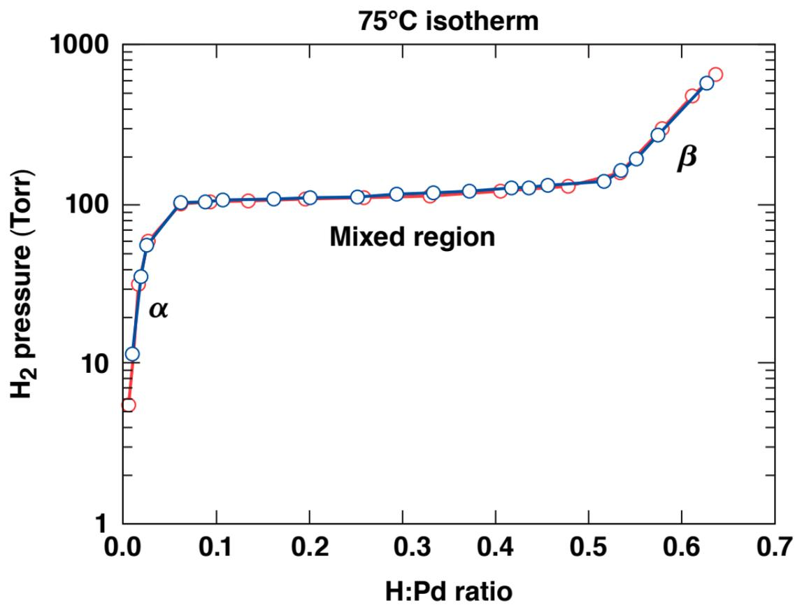
Figure 6: Two isotherms generated at 75° C to demonstrate reproducibility.
