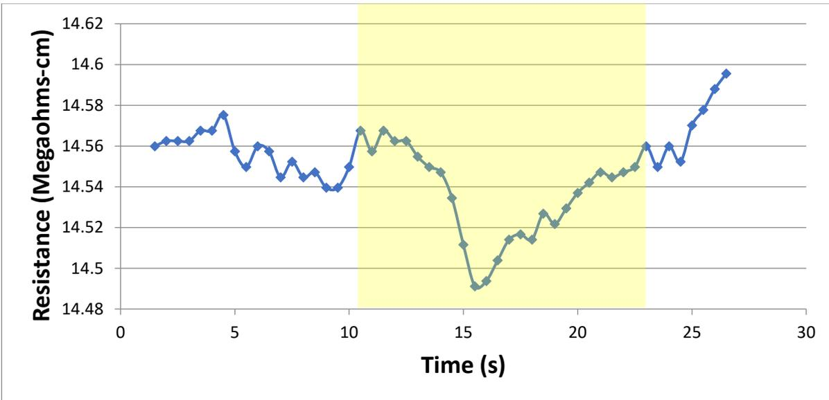
**Figure 17:** A graph of resistance with a flow rate of 0.9 gal/min. The change occurs at 12.5 seconds. The new flash-lamp system at 200 V was used to conduct this test. The Pulse Forming Network trigger occurred at ten seconds. The yellow area highlights the drop induced by the pulse.
