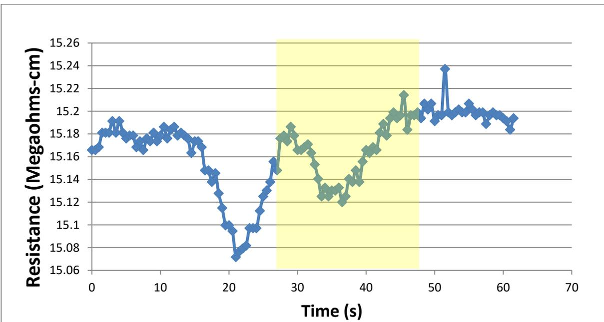
**Figure 16:** Data from sensor after contact with used flash-lamp system. There is a drop at 15.5 seconds followed by a second drop at 29 seconds. This test was conducted at 200 V. The Pulse Forming Network trigger occurred at ten seconds. The yellow area highlights the second drop induced by the pulse.
