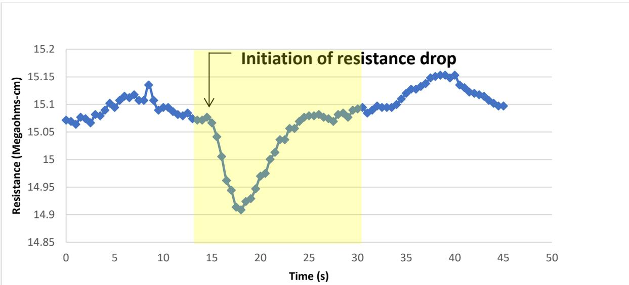
**Figure 11:** Typical plot of a used flash-lamp system test. The current is 6600 A. The voltage is 210 V. The plot illustrates a drop of approximately 0.16 Megaohms-cm. The pulse forming network trigger occurred at ten seconds. The yellow area highlights the drop induced by the pulse.
