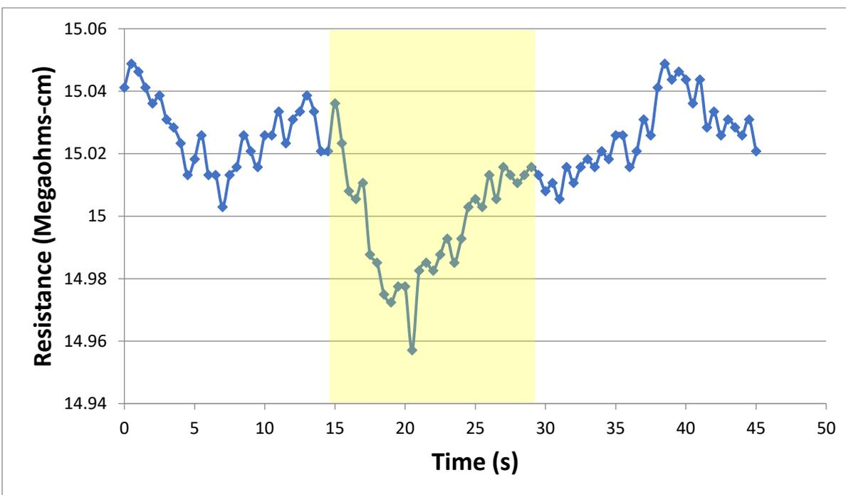
**Figure 9:** Typical plot of the cooling-water resistance as a function of time during a new flash-lamp system test. The current is 6700 A. The voltage is 210 V. A maximum drop of 0.061 Megaohms-cm was observed ten seconds after the pulse forming network trigger occurred. The yellow area highlights the drop induced by the pulse.
