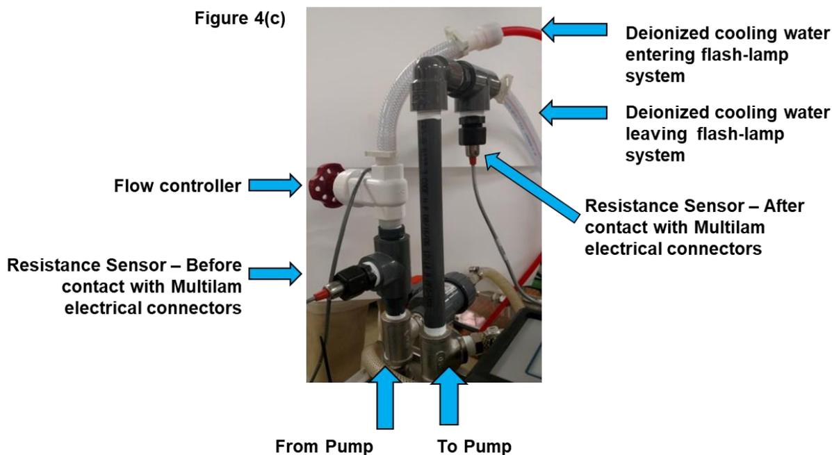
**Figure 4:** The entire experimental layout. (a) View showing the flash-lamp system. PFN: pulse forming network. (b) View showing auxiliary instruments of the PFN. (c) View showing the resistance sensors.
