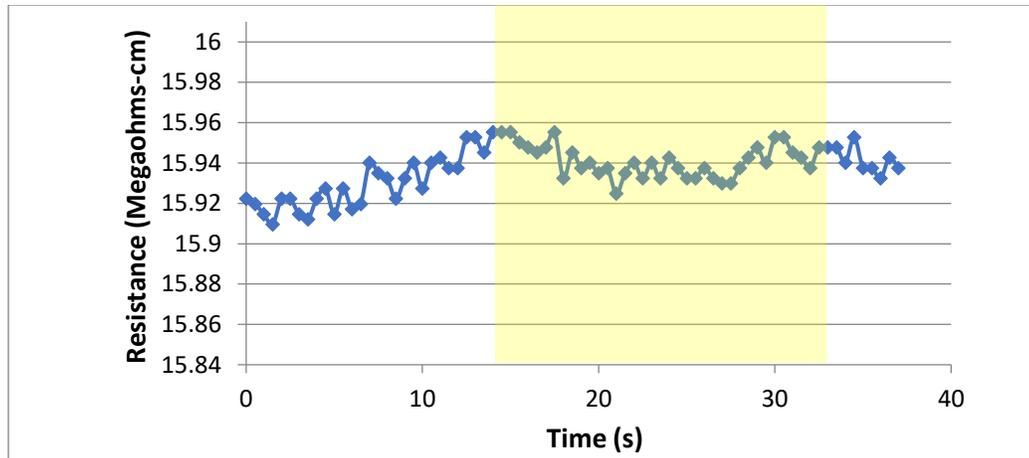
**Figure 10:** Typical plot of slightly used flash-lamp system test. The current is 5670 A. The voltage is 175 V. The graph illustrates a small change in resistance of approximately 0.02 Megaohms-cm. The pulse forming network trigger occurred at ten seconds. The yellow area highlights the drop induced by the pulse.
