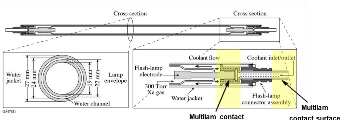
**Figure 6:** Cross sections of a flash lamp and its connector assembly. Highlighted yellow areas show Multilam contacts where deterioration in the flow of deionized cooling water can occur. Multilam bands are inside the female parts of connections. The male parts at these points, seen in the highlighted areas, incur deterioration.
