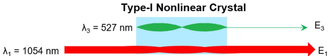
**Figure 3:** Illustration of the cascaded SHG process in a type-I nonlinear crystal, such as DKDP. The red beam represents the fundamental wave and the green beam represents its second harmonic.  $E_1$ ,  $\lambda_1$ , and  $E_3$ ,  $\lambda_3$  respectively represent the electric field amplitudes and wavelengths of the beams. For non-phase-matched conditions, periodic energy exchange occurs between the two waves, producing an intensity-dependent nonlinear phase shift in the fundamental wave.
