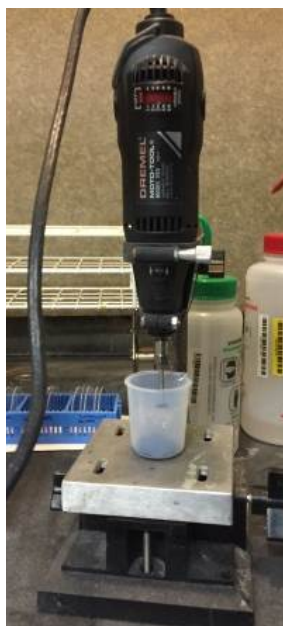
Fig. 8: Dremel Moto tool setup used for high-shear dispersion of absorbents into the oil samples.
