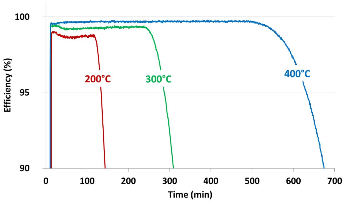
Figure 3.3 Dependency of gettingter efficiency on temperature
