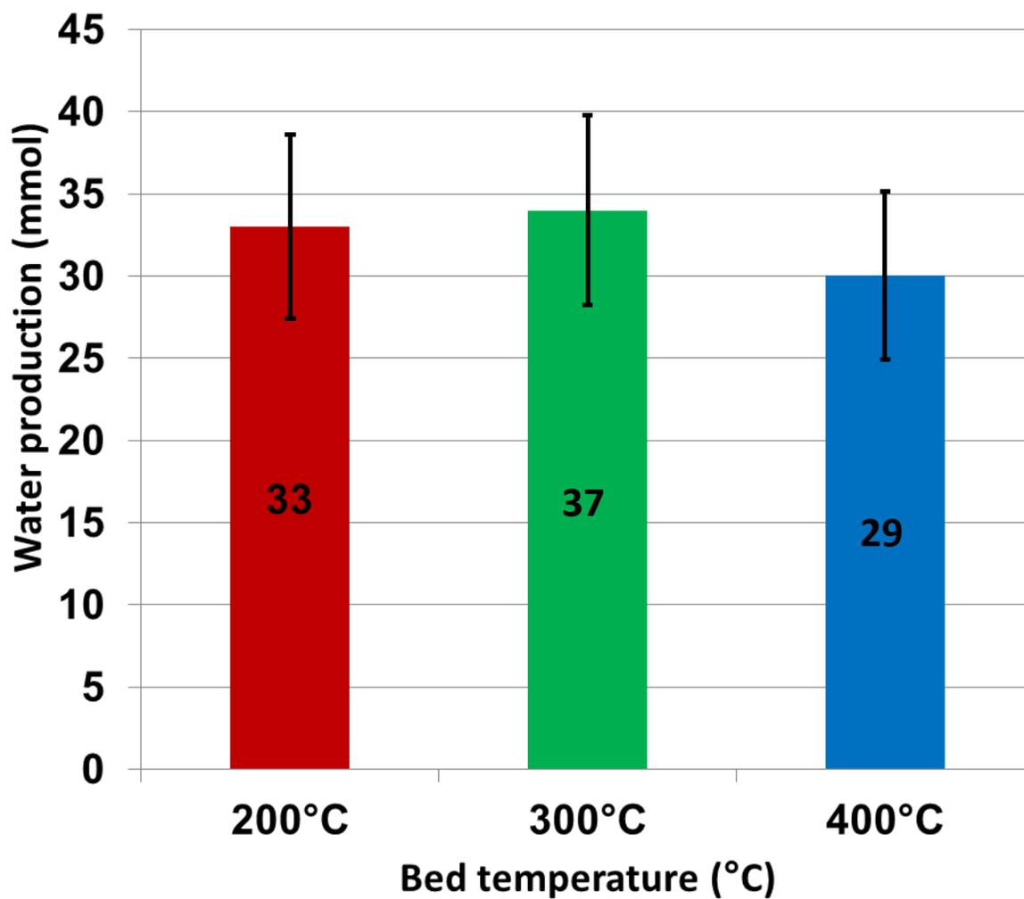
Figure 3.4 Dependency of water production on bed temperature
