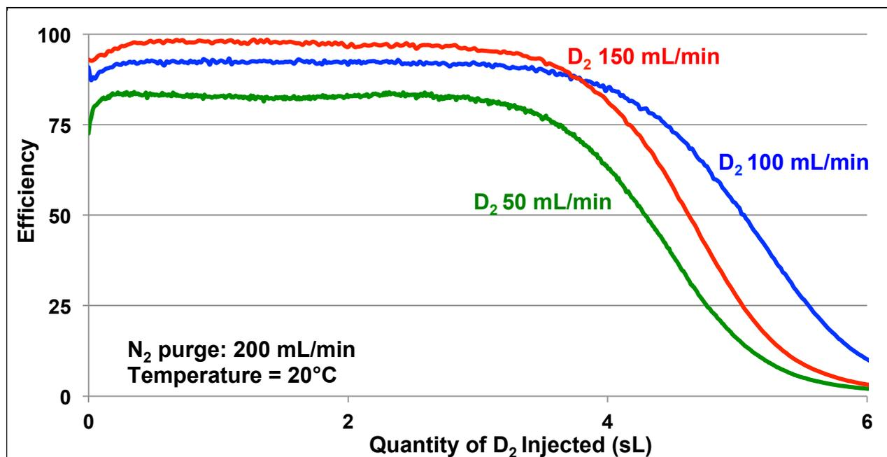
**Figure 5:** Displacement efficiency of  $D_2$  in a Pt/MS bed preloaded with  $H_2O$  as a function of the quantity of injected  $D_2$ , for three  $D_2$  flow rates. The curve for 100 ml/min matches the red curve of Fig. 4 (note the different horizontal scale).
