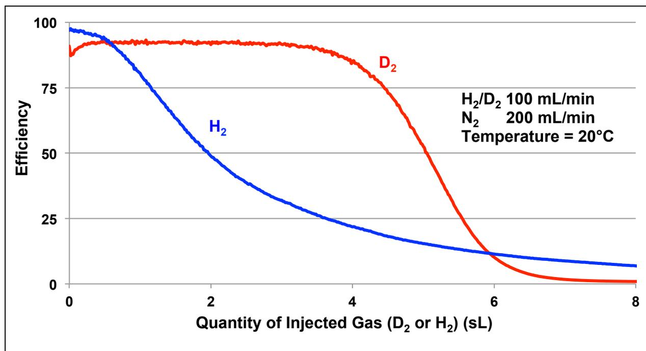
**Figure 4:** Red curve: displacement efficiency with which injected  $D_2$  is captured in a Pt/MS bed preloaded with  $H_2O$ , as a function of the quantity of injected  $D_2$ . Blue curve: same for injected  $H_2$  and a bed preloaded with  $D_2O$ .
