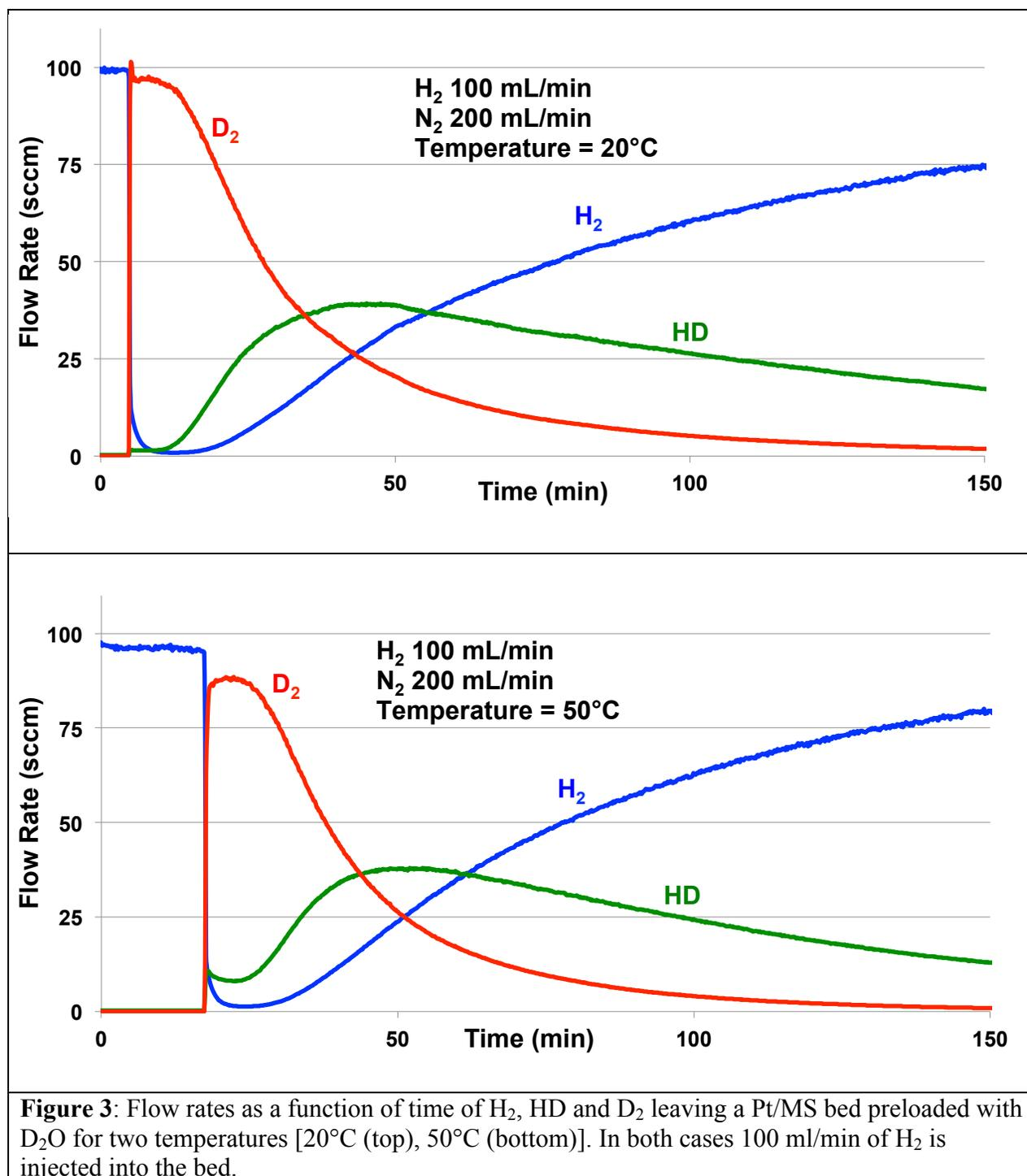
The displacement efficiency, defined as the percentage of the injected gas that is captured in the Pt/MS bed, is quantified in Fig. 4, which is obtained by integrating data shown in Figs. 2 and 3 with respect to time. Fig. 4 compares the displacement efficiency using either D<sub>2</sub> or H<sub>2</sub> as
