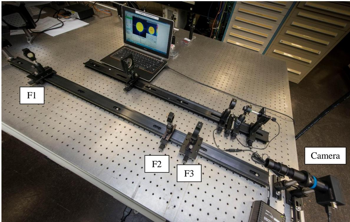
**Figure 7:** Lab setup of the three-lens system. The second and third lenses are on adjustable sliders. The system totals 1.4 m in length; however, note that due to table room constraints, the beam is bent in order to fit the system. The photo is taken by Eugene Kowaluk.
