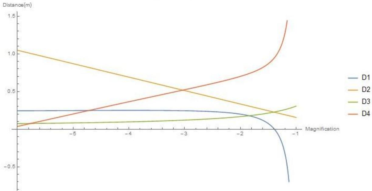
**Figure 3:** Graph of lens position (D1, D2, D3, D4) versus magnification.  $F1 = 200$  mm,  $F2 = -223$  mm,  $F3 = 250$  mm,  $L = 1.4$  m. Note that the graph of D1 is relatively flat across a wide range of magnifications while the graphs of D2, D3, and D4 are more variable.
