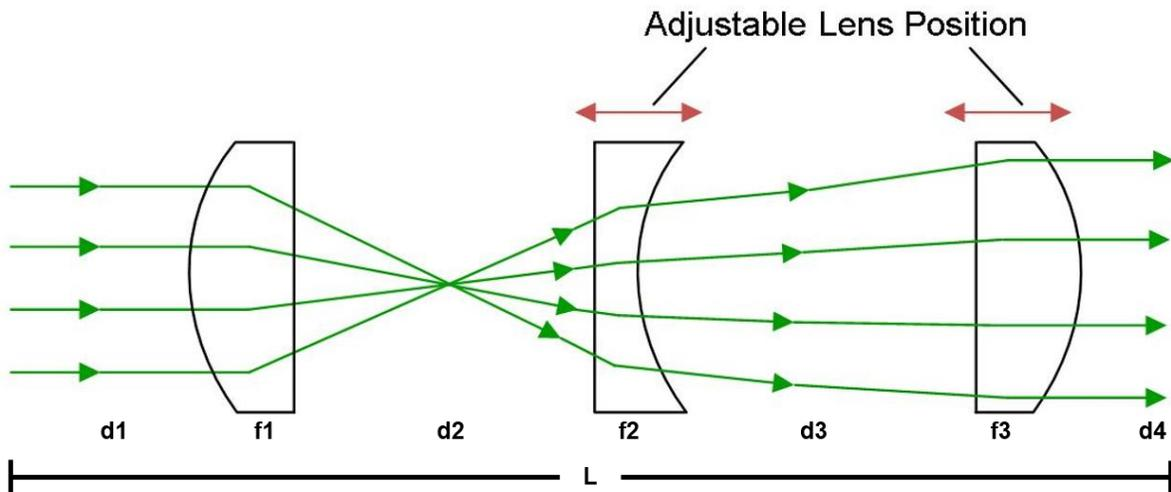
**Figure 2:** Schematic of the propagation of a beam through the proposed three-lens system. The first lens, F1, is fixed, and F2 and F3 are adjustable. The total length of the system, L, is also fixed. The ray paths are shown schematically; in reality the ray paths are refracted outward by the center lens F2.
