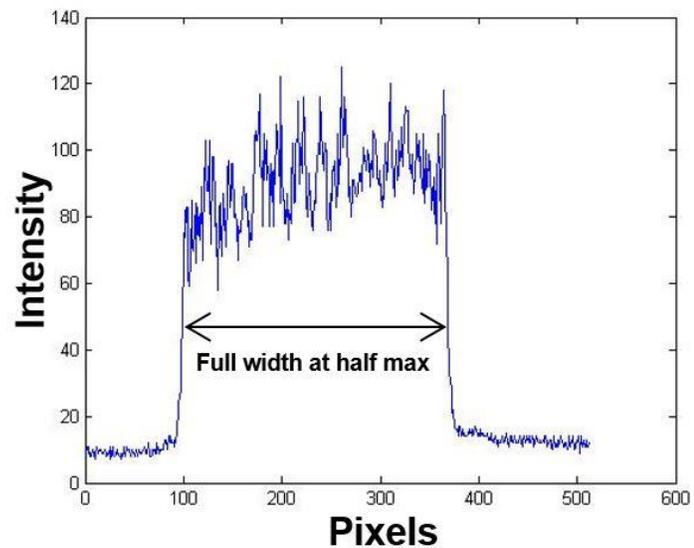
**Figure 9:** Lineout of intensity versus pixels at a magnification of -4. The full width at half max, the difference between the values of the independent variable at which the dependent variable is equal to half of its maximum value, is shown on the graph.
