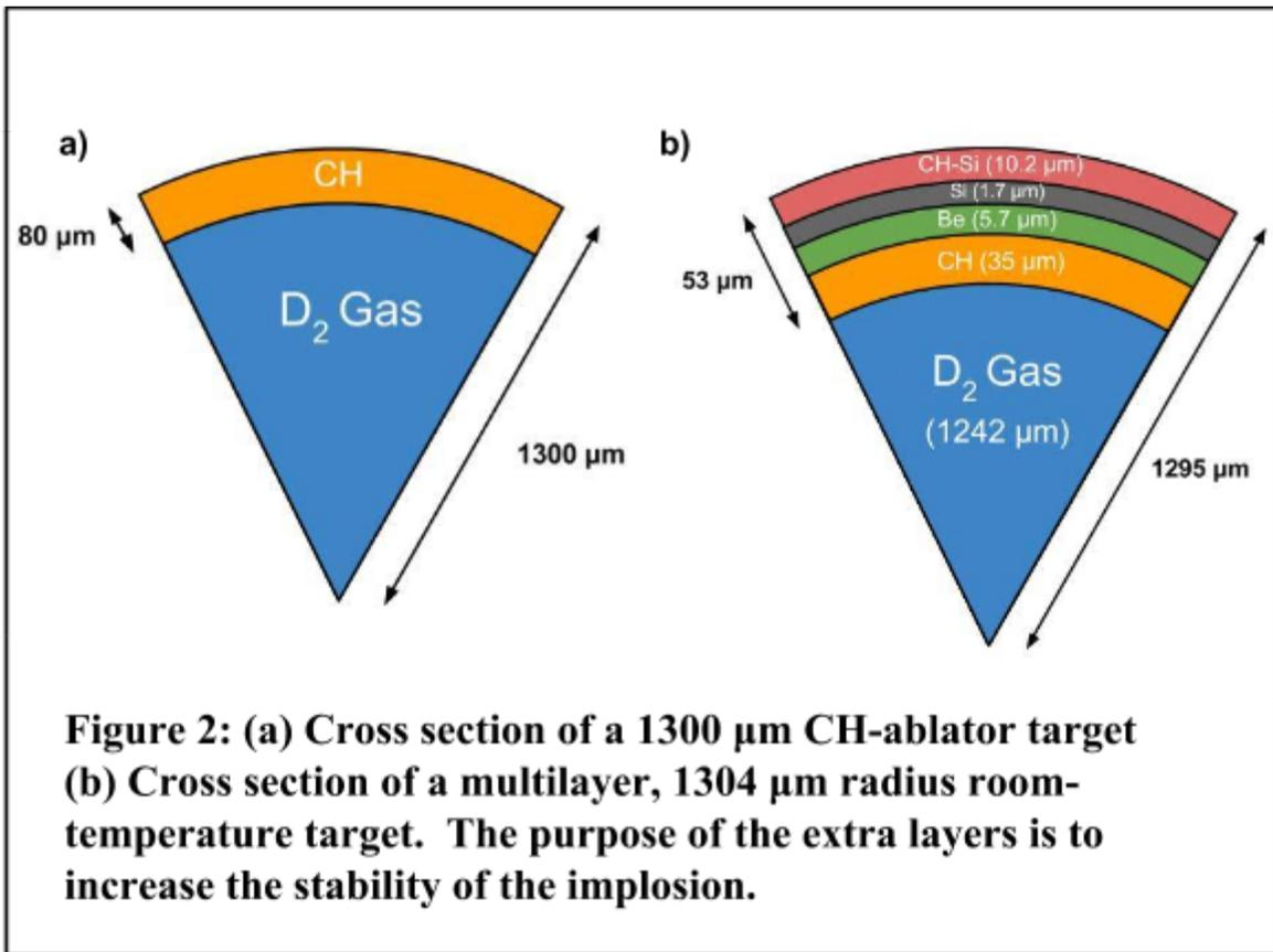
serves as a surrogate for the cryogenic layer. A surrogate target can be imploded more easily on the NIF as it does not require the hardware necessary for cryogenic implosions. This target design can therefore be used to study the physics of the implosion without actually imploding cryogenic targets. In an ignition-relevant implosion experiment, the inner CH shell would be replaced with cryogenic deuterium-tritium ice.
