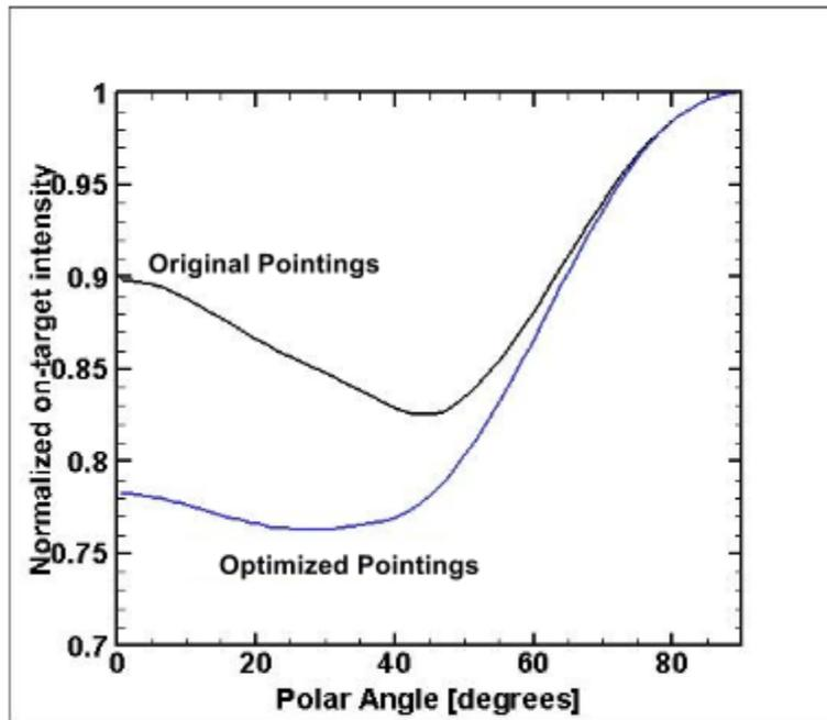
**Figure 4. Initial normalized on-target intensity at 0 ns for an implosion with original beam pointings and the on-target intensity at 0 ns for an implosion with optimized pointings.**
