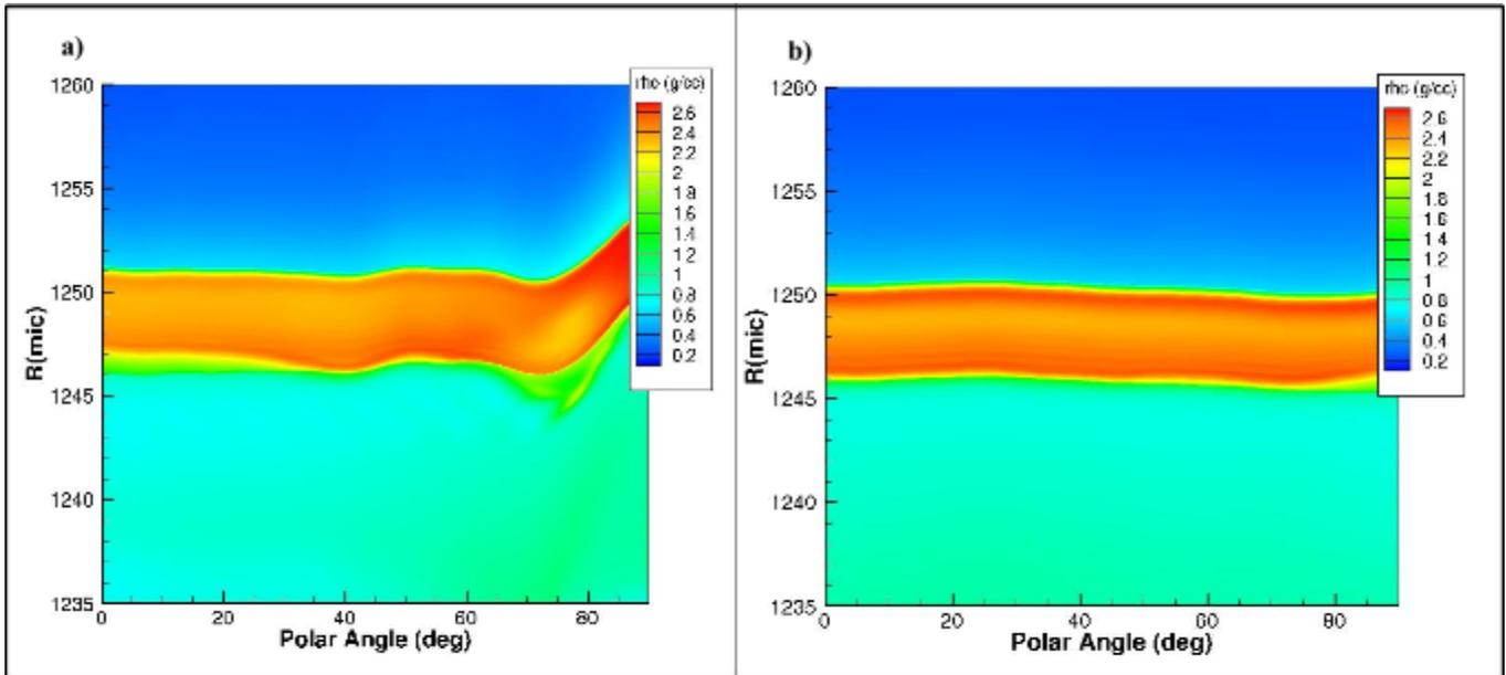
**Figure 6. (a) Density contours of multi-layer target with original pointings and beam power ratios at the time of third shock breakout. (b) Density contours of multi-layer target with optimized pointings and beam power ratios at the time of third shock breakout.**
