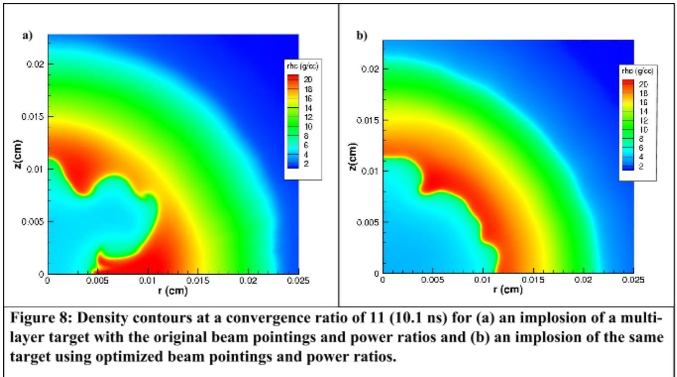
inner fuel-shell interface from the average radius of the interface and can be used as a quantitative measure of nonuniformity of the compressed core. In Fig. 8a, the hot spot distortion is calculated to be 8.5%, while the hot spot distortion of Fig. 8b is 3.9%. This
