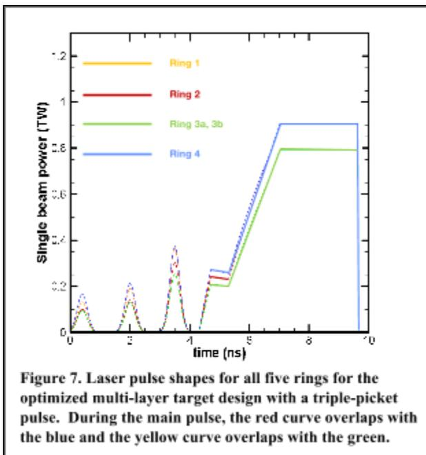
**Figure 7. Laser pulse shapes for all five rings for the optimized multi-layer target design with a triple-picket pulse. During the main pulse, the red curve overlaps with the blue and the yellow curve overlaps with the green.**
