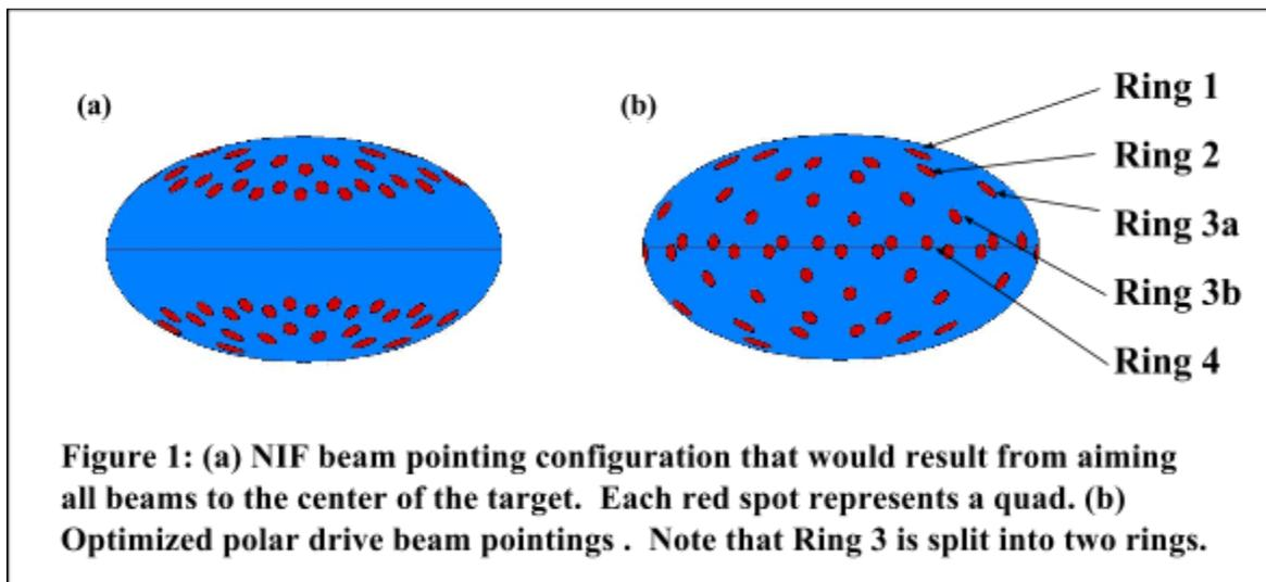
beams are shifted from their original normal angle of incidence, the repointed beams strike the surface of the target at more oblique angles of incidence. This results in the laser energy being deposited over a wider area of the target surface at more oblique angles, which equates to a reduction in drive.
