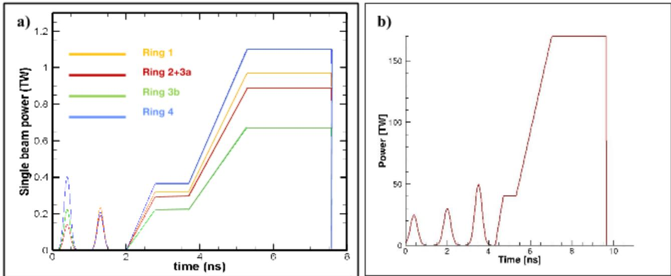
**Figure 3. (a) The double-picket pulse shape for the CH-ablator design showing the beam power in terawatts for each ring. Note that Rings 2 and 3a have identical pulse shapes. (b) The base triple-picket pulse shape used in this work, with the power summed over all 192 beams.**
