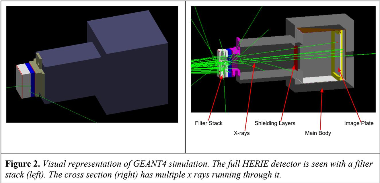
Figure 2 also shows visuals from a simulation with multiple beams running through the detector. Each beam of energy has the possibility of deflecting from, passing through, or being absorbed into each layer of matter it encounters. GEANT4 handles every interaction and ultimately determines how much energy was absorbed in the sensitive layer.
