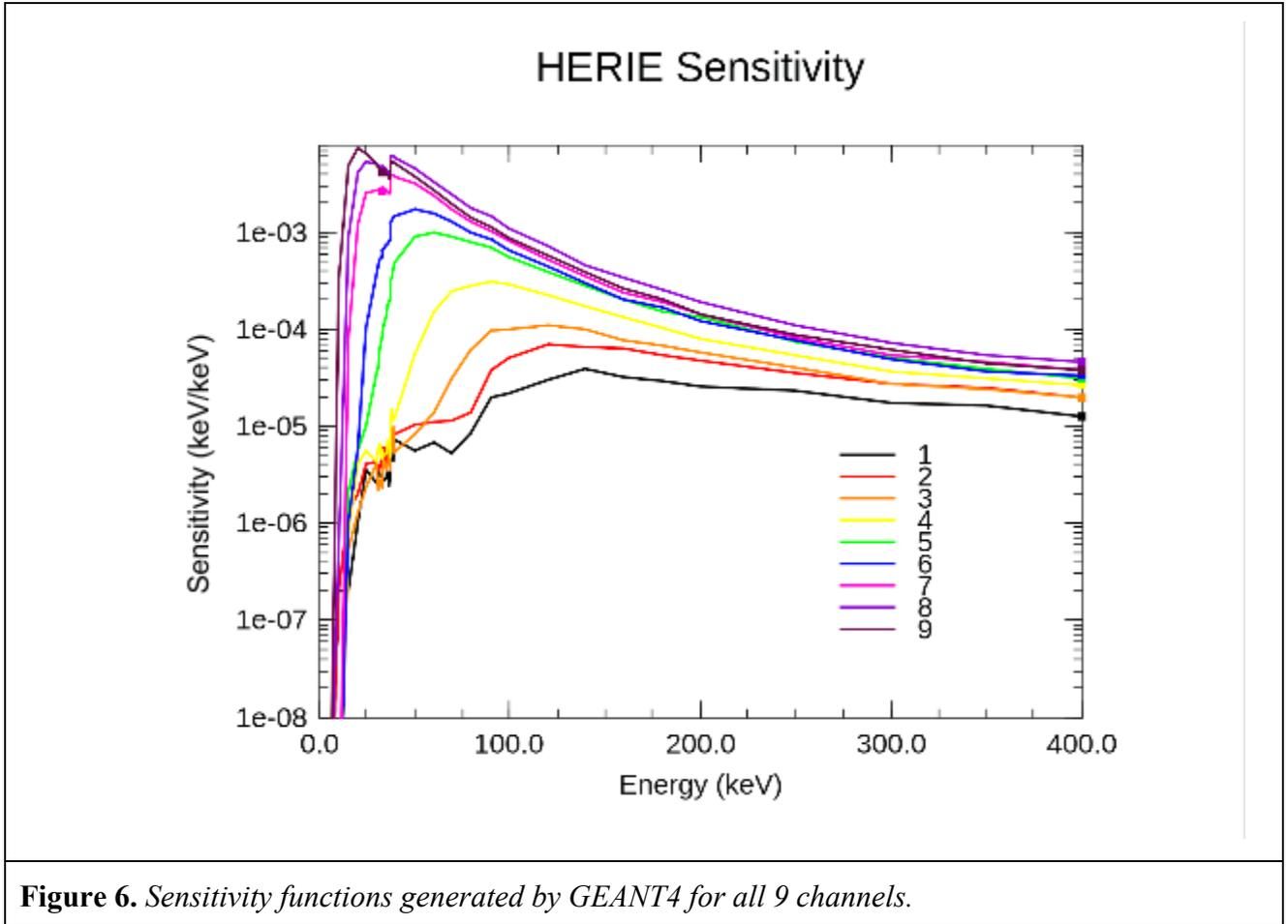
The combination of the functions shown in Figure 6 with the x-ray spectrum emitted by the target gives the total energy deposited in the image plate, which can be compared to the data collected during an experiment. The x-ray spectrum emitted from the target can be approximated by an exponential function of energy
