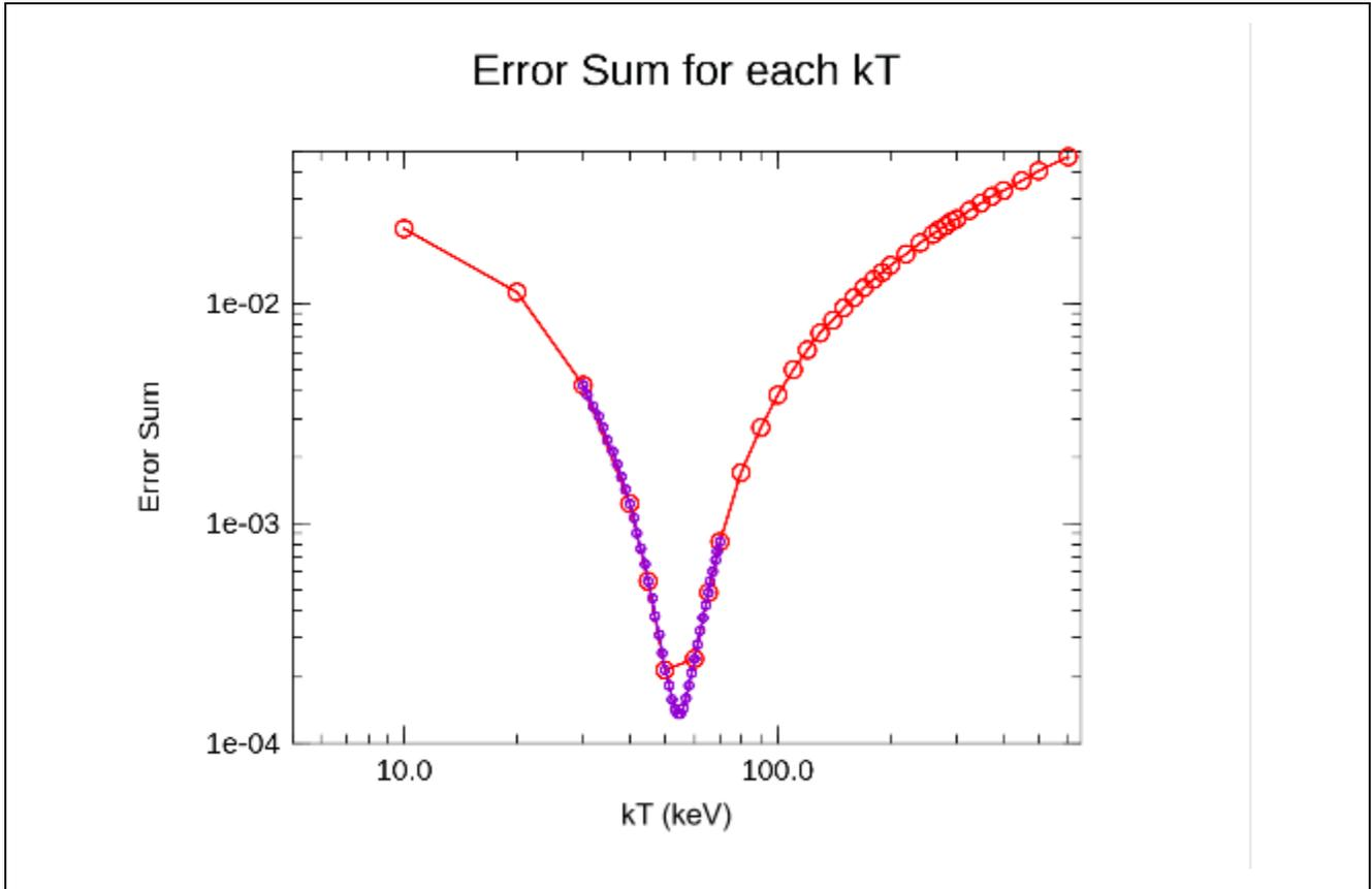
**Figure 7.** Error sum for a sample spectrum. The red model uses larger increments as a function of slope parameter  $kT$  to guess what the slope parameter  $kT$  is while the purple model uses smaller increments around the prediction of the red model to determine  $kT$  more precisely.
