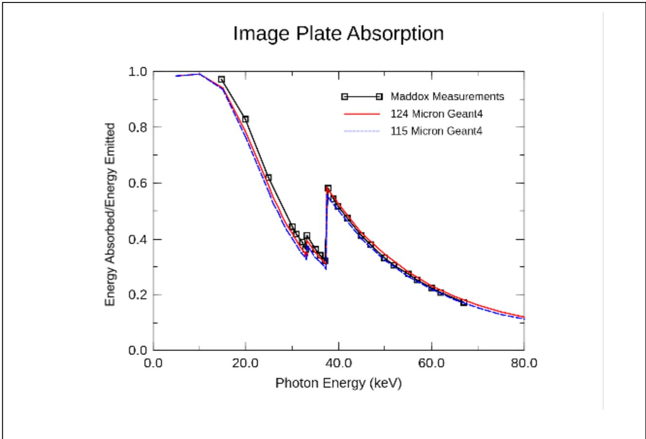
**Figure 3.** Graph of absorption functions for the image plate calculated by GEANT4 for image plate thicknesses of 124 and 115 microns. Published data from B. R. Maddox et al<sup>4</sup> are included.
