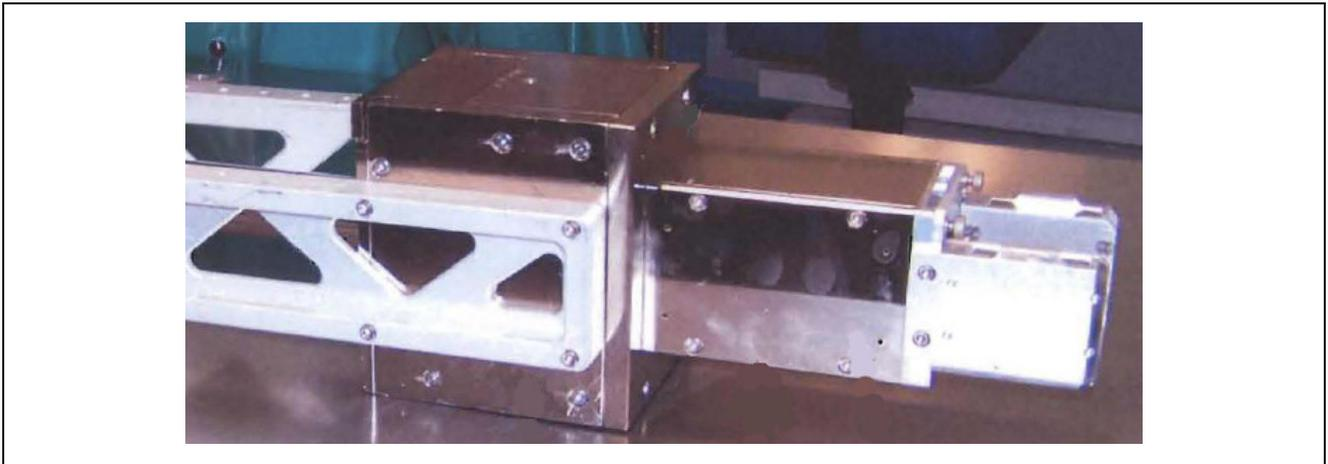
**Figure 1.** *Physical HERIE hard x ray detector*
