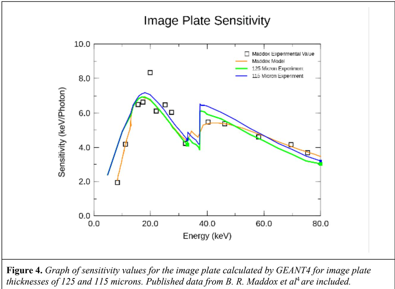
absorption edges found earlier. The difference between the two thicknesses appears larger in this test, but both are very close to the experimental data. The 125 micron thick plate was chosen for the rest of the simulations.
