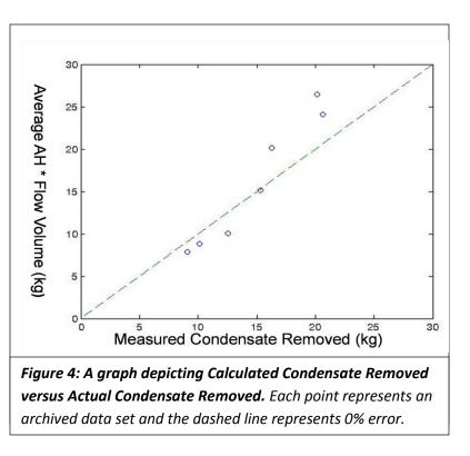
on some time intervals were overestimated or underestimated up to 30% deviation from the actual condensate removed, <u>Figure 4</u> indicates that using the average absolute humidity can provide a good estimate of the total condensate in the getter bed at any given time to within less than 30% deviation.
