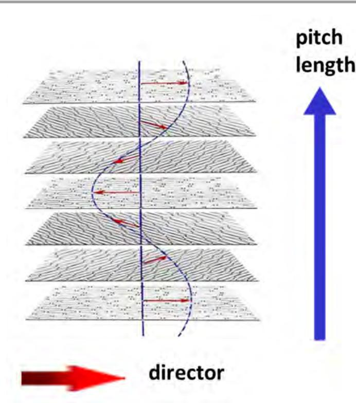
**Figure 1: A depiction of a chiral nematic LC. The director denotes the average orientation of the molecules in each layer. The pitch length is the distance required for the director to make a 360° rotation.**
