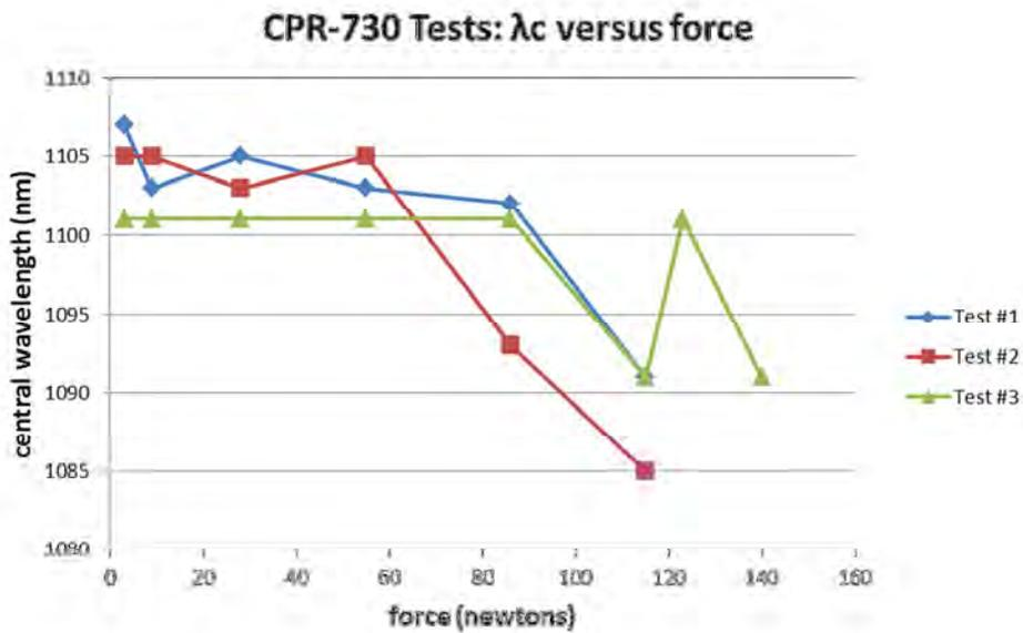
**Figure 7.** The correlation between  $\lambda_c$  and force applied to CPR-730 for all three pressure tests. It seems that as pressure was increased, the gap thickness and  $\lambda_c$  decreased. It is believed that the outlier at ~125 N was caused by inaccuracy of the transmission scan.
