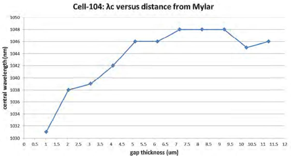
**Figure 5. Central wavelength,  $\lambda_c$ , of a wedged cell (Cell-104) as a function of gap thickness. As the distance from the spacer increased, the gap thickness decreased, and the  $\lambda_c$  decreased.**
