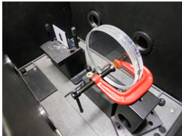
**Figure 6. (a) Approximate newtons applied to the CPRs. (b) CPR-730 and clamp in the Lambda-900 testing chamber.**
