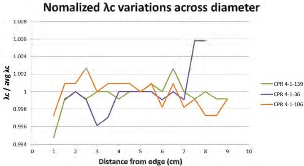
**Figure 4. The central wavelengths,  $\lambda_c$ , of three of the scanned CPRs. There are variations in  $\lambda_c$  across the diameters of these CPRs.**
