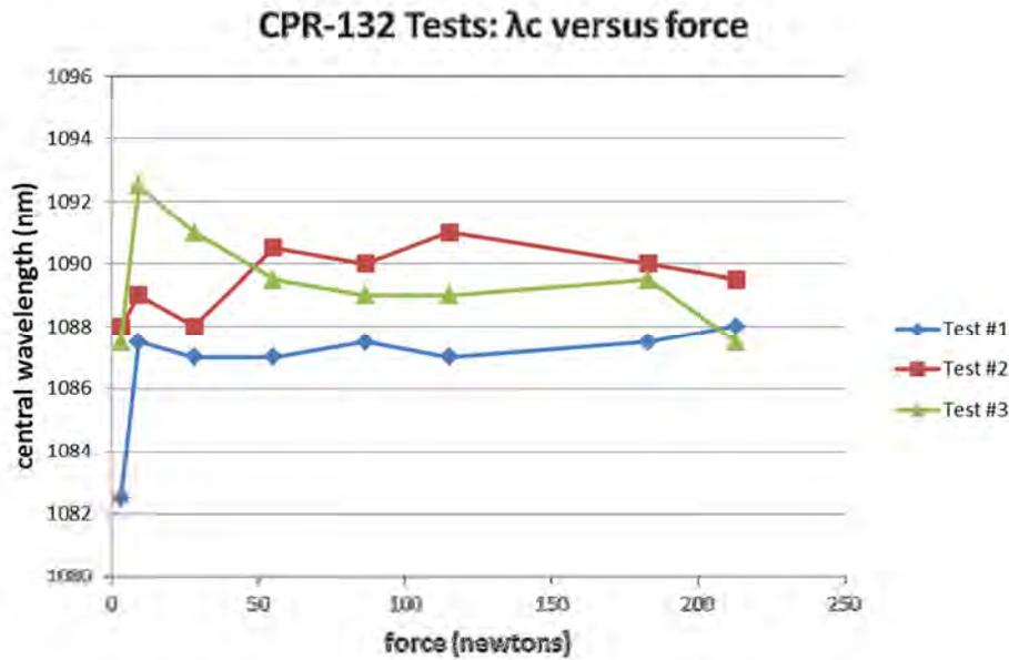
**Figure 8. The central wavelengths and force applied to CPR-132 for all three pressure tests. In contrast to Figure 7, no clear correlation is seen between applied pressure and  $\lambda_c$ .**
