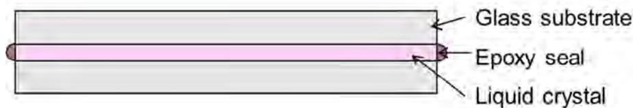
**Figure 2.** LCPs consist of two glass substrates, a thin layer of chiral nematic LC fluid, and an epoxy seal. The LCPs are filled at an elevated temperature, cooled to room temperature, sheared, and sealed.
