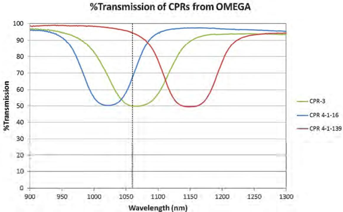
**Figure 3. The percent transmission (% T) of three CPRs from the OMEGA system. Because the spectrophotometer emits equal amounts of right and left circularly polarized light, 50% transmission indicates that the CPRs are reflecting the correct amount of light. The dotted line indicates the specified  $\lambda_c$  at normal incidence (1060 nm). CPR-3 is performing well, but CPR 4-1-16 and CPR 4-1-139 have shifted to the blue and red, respectively, and are ineffective polarizers at 1060 nm.**
