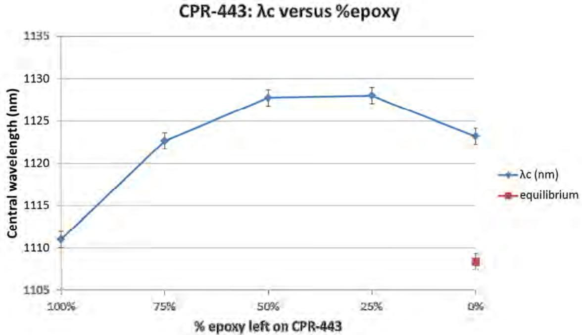
**Figure 10.** The  $\lambda_c$  increased as epoxy was removed and air bubbles entered the gap between the substrates.
