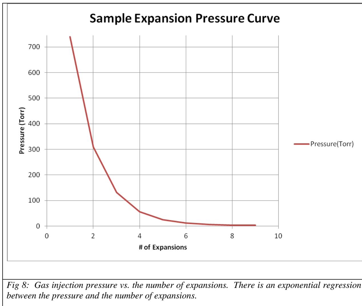
Since the pressure transducer measuring sample pressure attached to the GC can only read up to 1000 torr, the instrument can't read a 5000 torr gas sample. As a result, multiple expansions had to be made in order to bring the pressure down to a readable pressure. An expansion is performed when the sample gas is first injected into the GC, and then placed under
