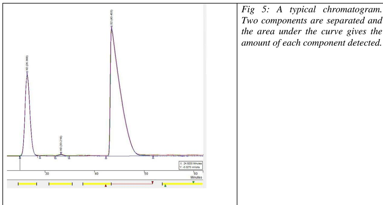
*Fig 5: A typical chromatogram. Two components are separated and the area under the curve gives the amount of each component detected.*
