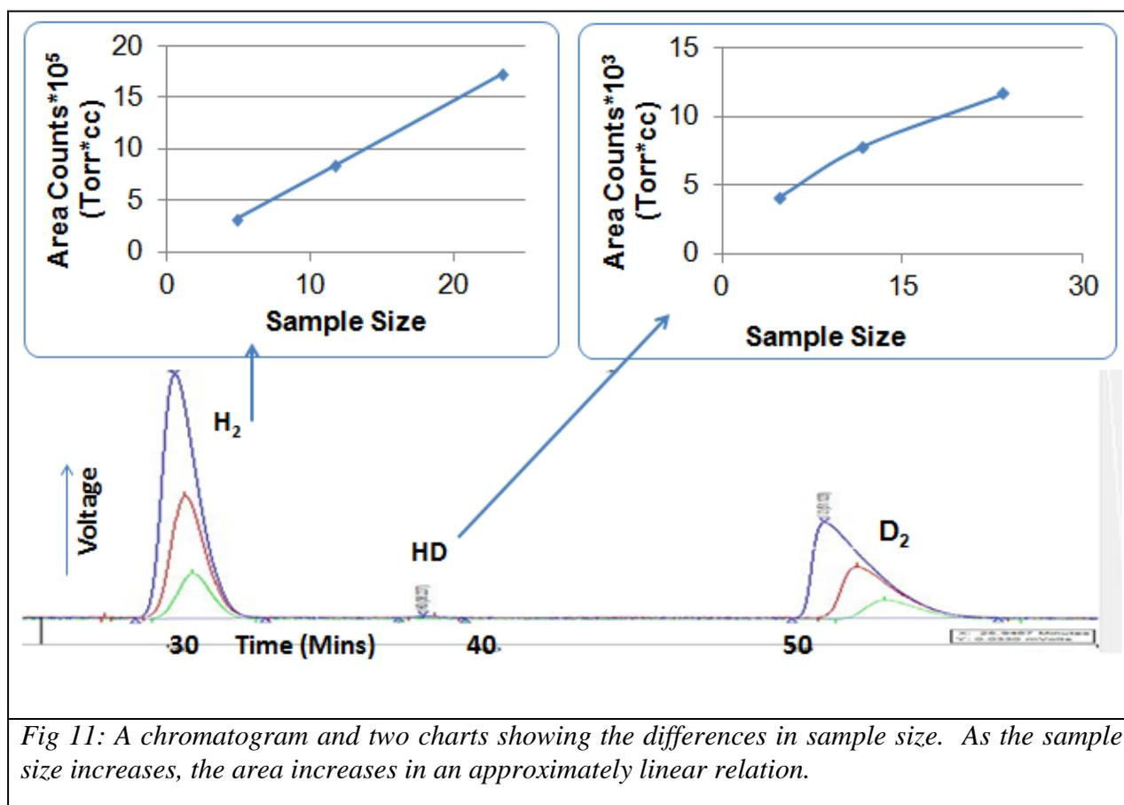
Figure 11 shows three chromatograms with different sample sizes and a different number of expansions. A sample size refers to how much sample is injected into the GC. As more expansions are made, the sample size decreases. The green chromatogram represents 6 expansions, while the red and blue chromatogram represents 5 expansions and 4 expansions, respectively.
