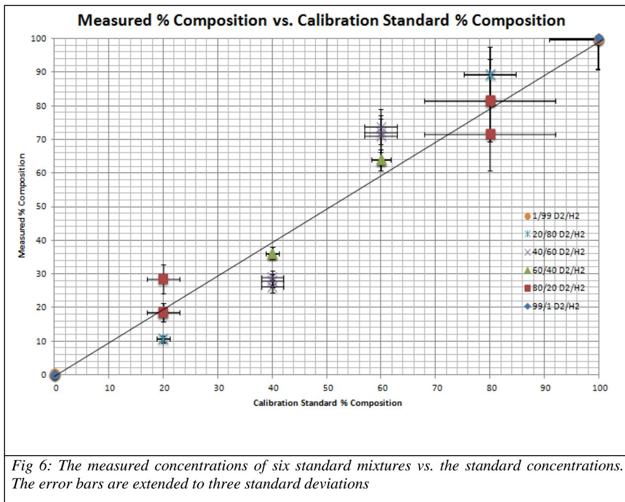
As seen on figure 6, most of the mixed concentrations don't match the measured concentrations. For example, the standard created at 40/60%  $H_2/D_2$  was measured by the GC at 36%/64%  $H_2/D_2$ . In addition, even with the error bars at 3 standard deviations, the measured amounts don't match the mixed standard. The y error bar is three times the rms of the three runs.
