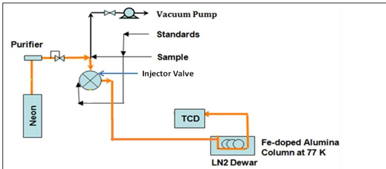
*Fig 2: Schematic of the GC setup. The GC comprises the alumina column and the TCD. The injector valve allows different gases to flow into the GC. The orange arrows represent the carrier gas flowing through the GC.*
