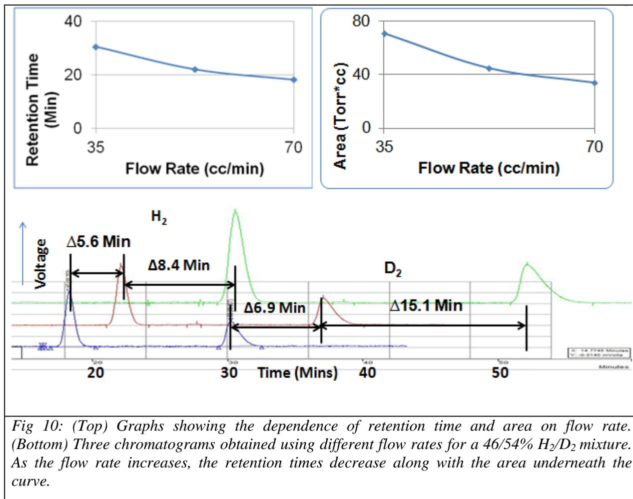
Fig 10: (Top) Graphs showing the dependence of retention time and area on flow rate. (Bottom) Three chromatograms obtained using different flow rates for a 46/54% H<sub>2</sub>/D<sub>2</sub> mixture. As the flow rate increases, the retention times decrease along with the area underneath the curve.
