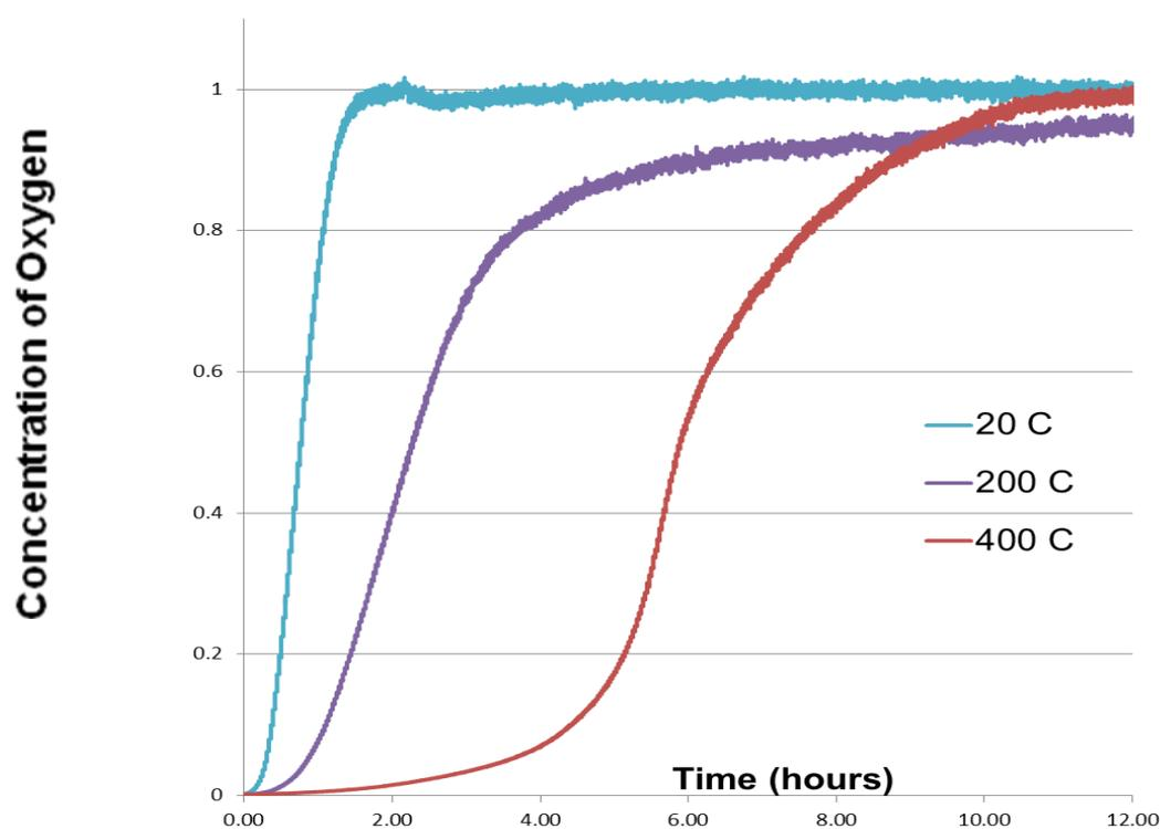
The evolution of the oxygen concentration in the carrier leaving the bed is illustrated in Figure 3.2 for three different operating temperatures. The carrier flow rate is fixed at 2 L/min and
