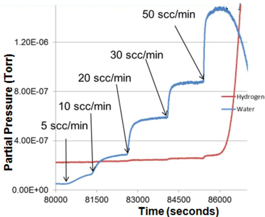
Figure 3.4 illustrates a typical regeneration at 500 °C using a helium purge rate of 2 L/min. As the hydrogen flow rate is increased from 5 scc/min to 50 scc/min the water partial pressure in the carrier at the bed outlet increases proportionately. Towards the end of the run, the water partial pressure is observed to drop and concomitantly the hydrogen partial pressure increases as the quantity of residual nickel oxide in the bed disappears.
