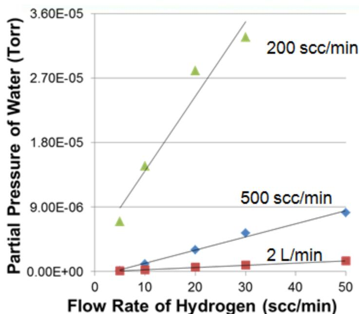
Figure 3.5 summarizes three regenerations at 500 °C for varying helium and hydrogen flow rates. At a helium purge rate of 500 sccm and 2 LPM, the partial pressure of water appears to increase linearly with increasing hydrogen flow rate (or partial pressure). For a helium purge rate of 200 sccm, the water production rate deviates from linearity and appears to approach a saturation value that is independent of the hydrogen partial pressure in the carrier.
