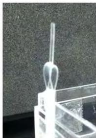
*Figure 2: Pictures of sample preparation setup, materials, and completed sample. a.) The chemistry clamp holds the polystyrene strip, while the polystyrene loop is attached to the blue lab jack. The entire setup is placed in front of the Green Spot light source for immediate curing. b.) This is a completed sample.*
