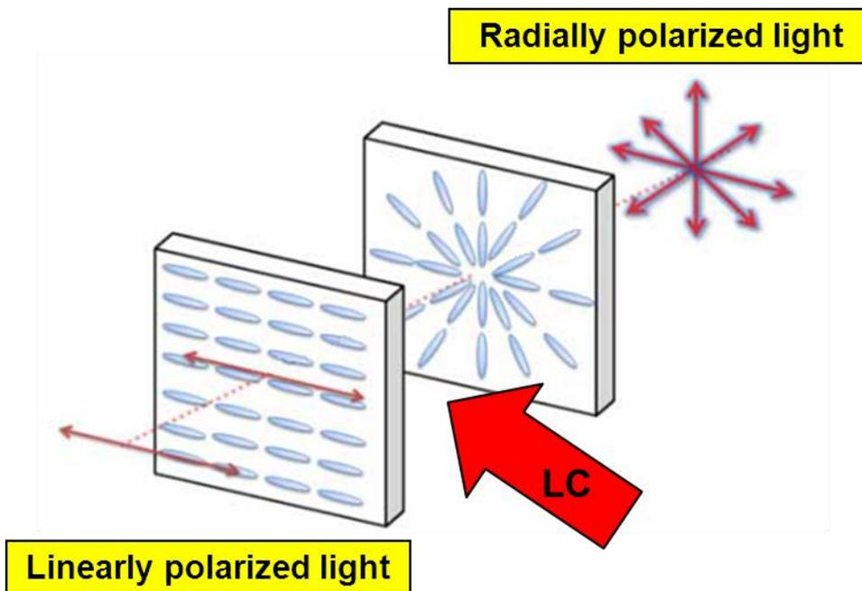
**Figure 1: Schematic of a radially polarizing LC device. It consists of a linearly patterned substrate (left) and a radially patterned substrate (right), put together and filled with a twisted nematic liquid crystal**
