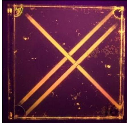
**Figure 4: (a): Artifact found in center of devices with unaligned slit and rotating-stage. (b): A calibration cell. 3 lines at 3 discrete angles ( $45^\circ$ ,  $135^\circ$ , and  $225^\circ$ ) were made using the slit in the rotating-stage setup. Proper alignment of the rotation axis and slit produces only two lines. Viewed through crossed polarizers.**
