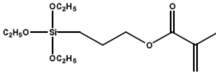
Fig. 2: 3-Methacryloxypropyltriethoxysilane (MOTOS). The carbon-carbon double bond (vinyl group) on MOTOS provides an opportunity for a crosslinking agent to create bonds between  $\text{SiO}_2$  particles
