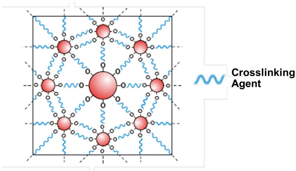
Fig. 3: Modified, crosslinked silica oxide particle. The silica oxide particles have been modified, allowing the crosslinking agent to create bonds between particles forming a robust network.
