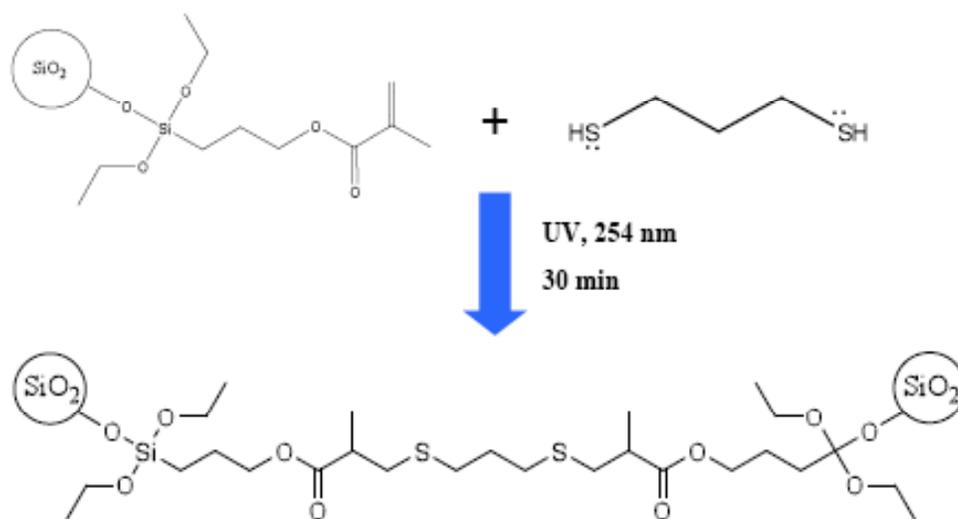
Fig. 4: Photoinitiated crosslinking reaction. The nucleophilic dithiol (propanedithiol) reacts with two different modified SiO<sub>2</sub> particles, forming a network of bonds between SiO<sub>2</sub> particles.
