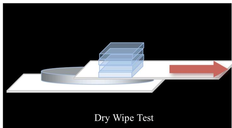
Fig. 5: Dry wipe test diagram for abrasion resistance of a coating. The top clean-room wipe carrying a stack of substrates was dragged in a straight line across the surface of the coated substrate, which was then observed with the naked eye for any scratches.
