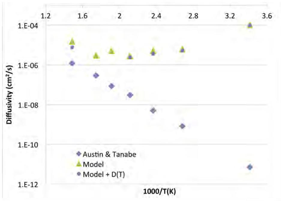
Figure 5. Plot of the tritium diffusion coefficient dependence on temperature of stainless steel
