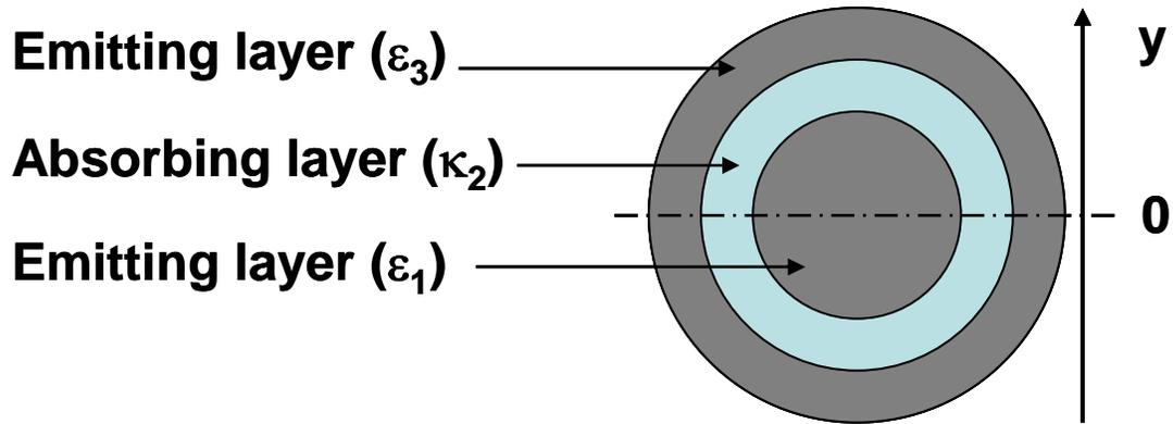
Fig. 1 The target is modeled with an emitting layer surrounding an absorbing layer, all surrounding an emitting core.
