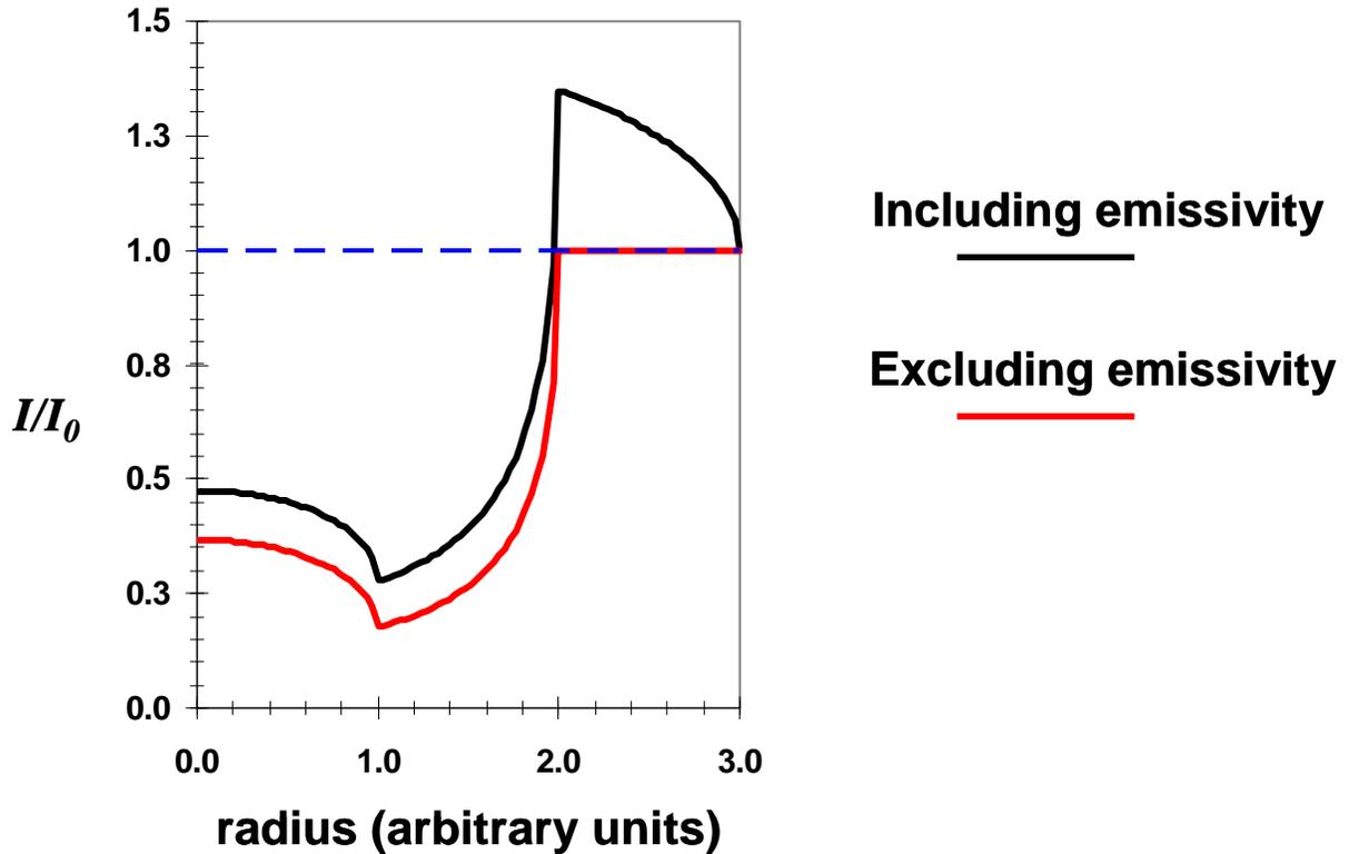
Fig. 3 Radial optical thickness profiles with and without including a strong, thick emitting outer layer.
