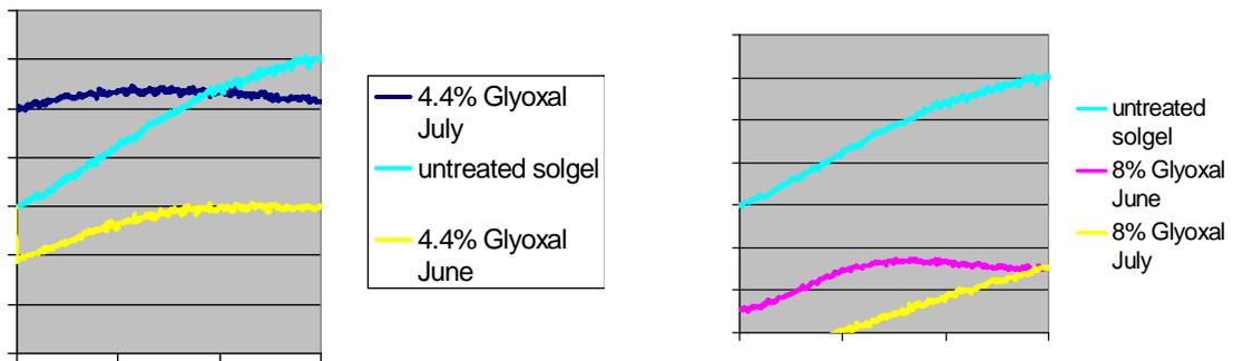
Fig. 8: Optical transmission of glyoxal-modified coatings as a function of aging time. *Left:* Coating modified with 4.4% wt glyoxal. *Right:* Coating modified with 8 wt% glyoxal. Transmission curves for a standard (non-crosslinked) sol-gel coating are included for reference.
