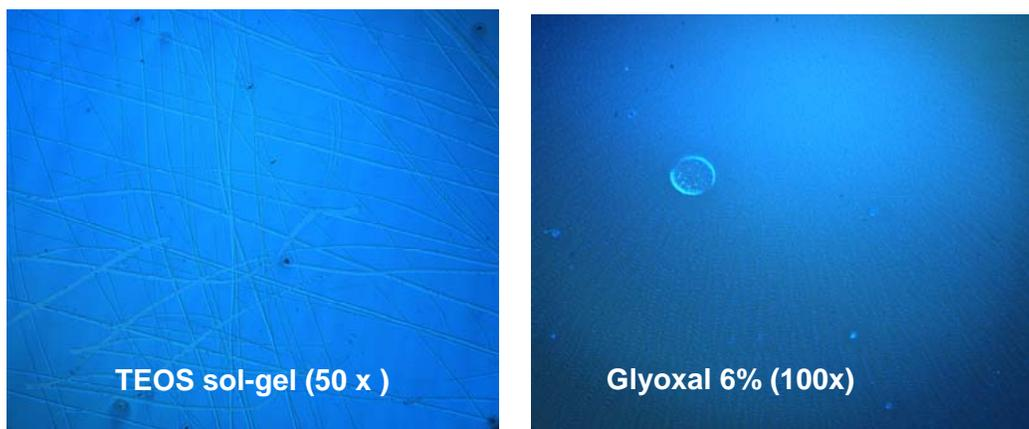
Fig. 6: *Top*: Abrasion resistance data for modified sol-gel coatings aged for 4 weeks. *Bottom*: Photomicrographs of standard TEOS sol-gel AR and 6% glyoxal-modified sol-gel AR after drag-wiping with 7.4 g and 160 g mass loads, respectively.
