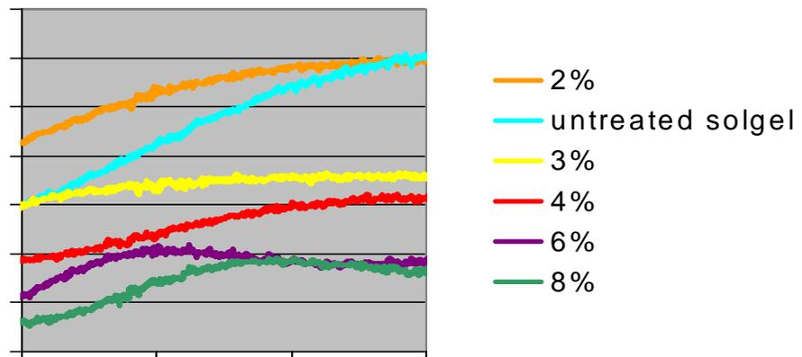
Fig. 7: Transmission spectra of modified sol-gel coatings as a function of cross-linking agent concentration. *Top*: Transmission spectra for acryloyl chloride-modified sol-gel coatings. *Bottom*: Transmission spectra for glyoxal-modified sol-gel coatings. Included with both sets of transmission spectra are a transmission profile for a standard (non-modified) sol-gel coating as a reference.
