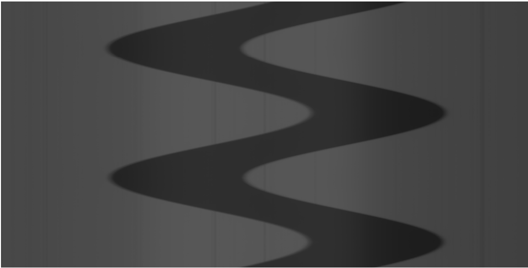
Figure 5: An example image taken with a line-scan camera of a vibrating target stalk mounted on a shaker table. The stalk itself is magnified to approximately 6 cm in width. The time axis is vertical.
