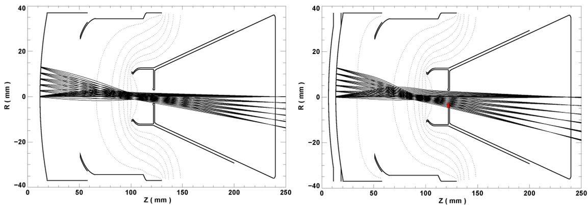
*Fig. 3: Ray traces for low field ( $V_{ks}=500\text{ V}$ ) and high field ( $V_{ks}=2500\text{ V}$ ) power supplies, respectively. More light reaches the cathode with an LFPS because more light is allowed through the anode aperture. The red line shows the part of the anode that blocks rays as a result of using the HFPS.*
