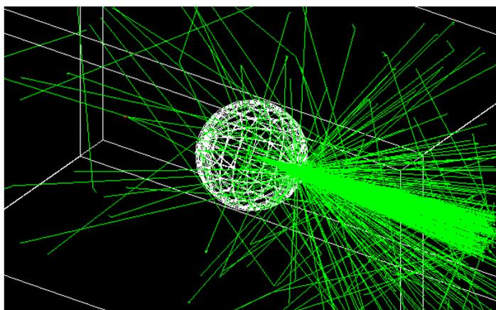
**Figure 6: Neutron Scattering – Neutrons (green) with directions within a cone (increased solid angle for visualization) are scattered by the target chamber. The majority of scattered neutrons are deflected by a small angle ( $< 45$  deg).**
