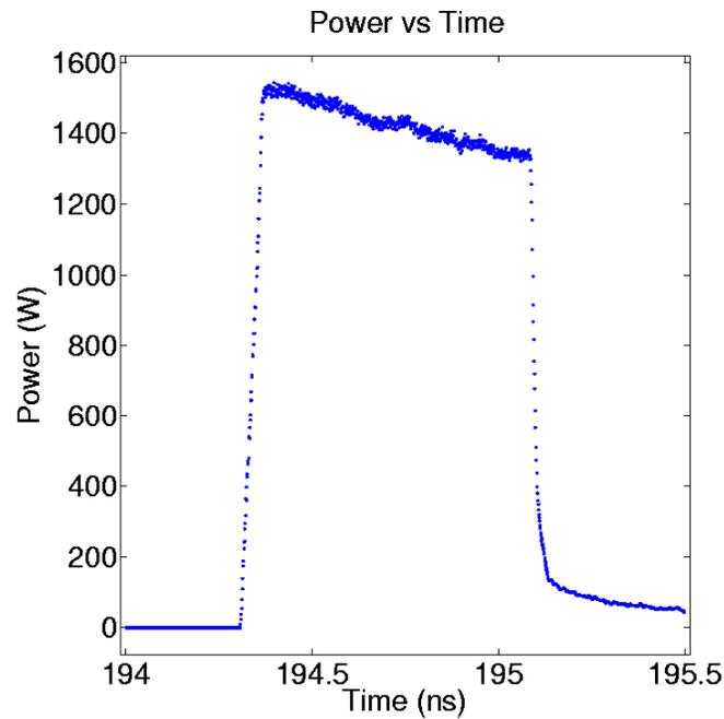
**Figure 4: First Test – Energy deposition signal for 14.1 MeV neutrons through a 4 cm detector placed 10 m away from the target. The sharp rise and drop of the signal correctly correspond to the times at which the non-interacting neutrons pass through the detector. Between these times, the signal drops off exponentially.**
