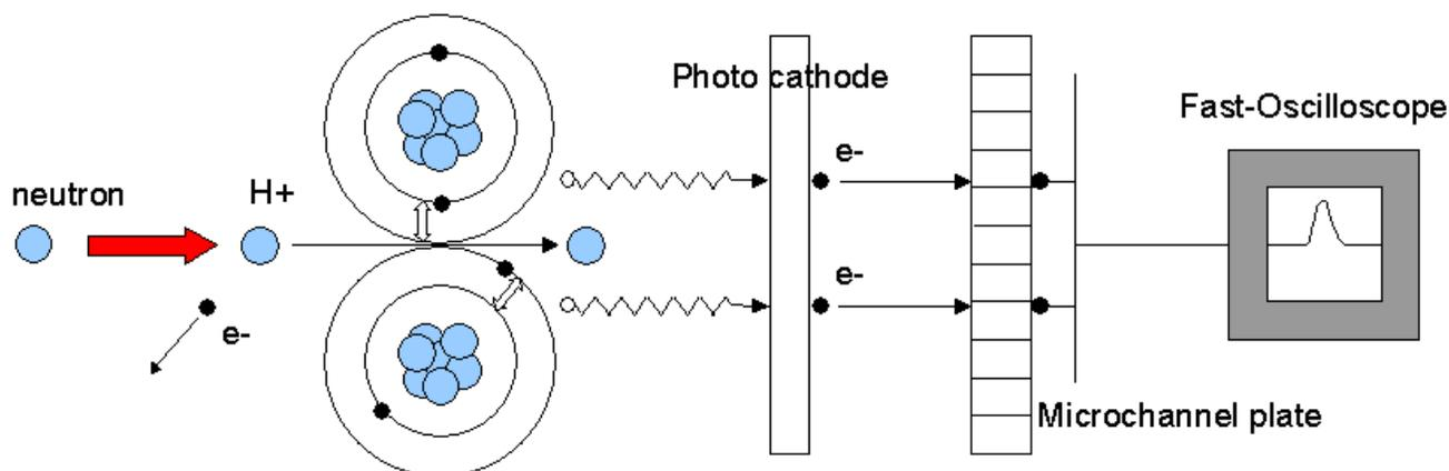
**Figure 1: Scintillation process – A neutron collides with the nucleus of an atom such as hydrogen. The atom becomes ionized and excites and de-excites nearby atoms, emitting photons. The photons generate current in a photocathode. The current is amplified by a microchannel plate and read by a fast oscilloscope.**
