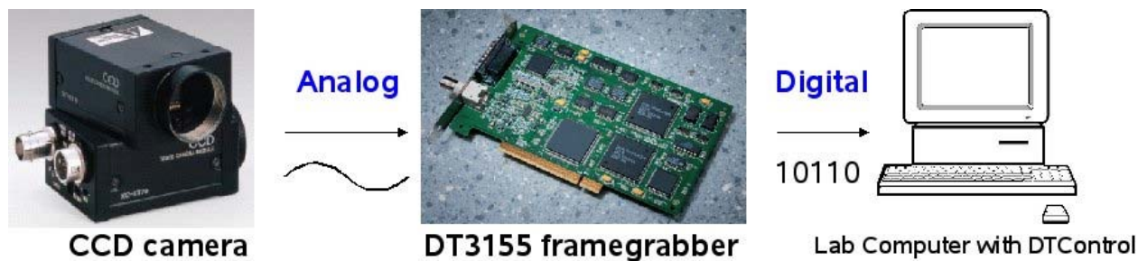
Figure 1.2: A CCD camera, DT3155 framegrabber and DTControl in use 2,3,4
