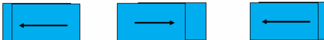
Figure 3.2- The shear method. Arrows show which way the top substrate slides over the bottom substrate.
