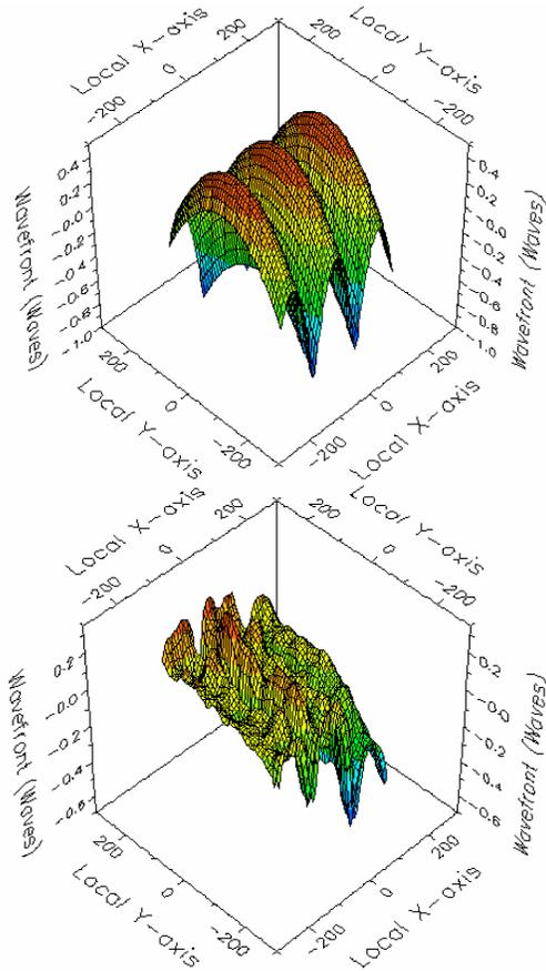
Figure 4 – **The DM corrects for the broadening of the pulse** – The upper image is the wavefront of the pulse when quarter-wave error is applied to the diffraction gratings. The lower wavefront shows the corrections of the DM in narrowing the pulse.
