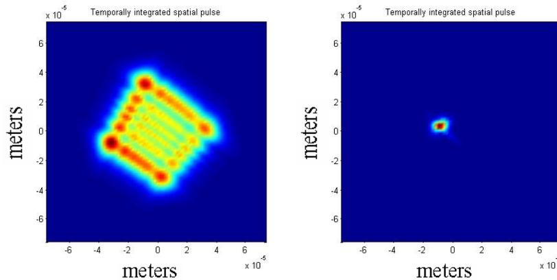
Figure 6 – **The DM is able to correct the encircled energy of the continuous curvature error to within the desired value** – The smearing evident on the uncorrected far field (left) is nearly eliminated when the DM is applied to the wavefront.
