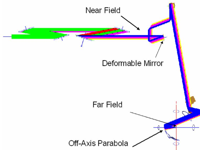
Figure 1 – **Modeling in FRED** – Beams are propagated through the pulse compressor to the deformable mirror and on to the off-axis parabola. The encircled energy and FWHM of the compressor are found at analysis planes in the near field and far field.
