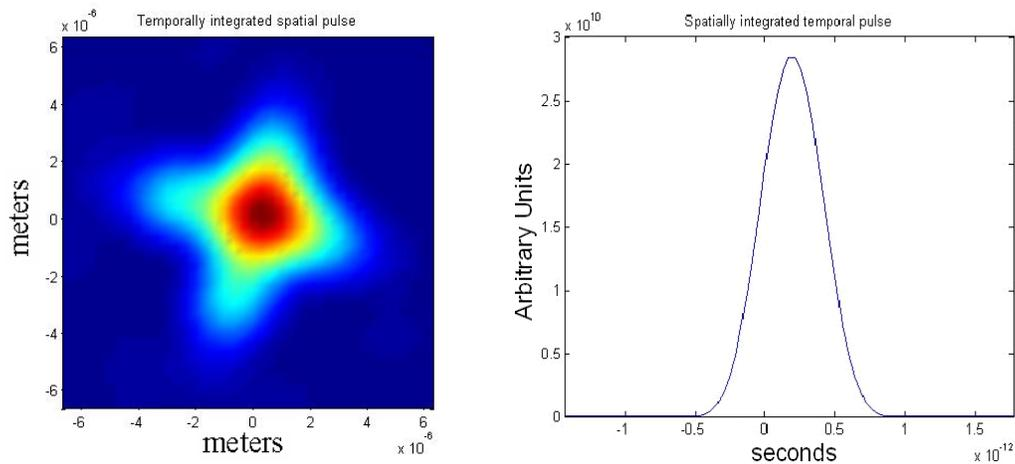
Figure 2 – **“Perfect” Compressor** – The encircled energy of the pulse of the “perfect” compressor may be viewed in the temporally integrated spatial pulse (left). The spatially integrated temporal pulse (right) shows the FWHM of the pulse.
