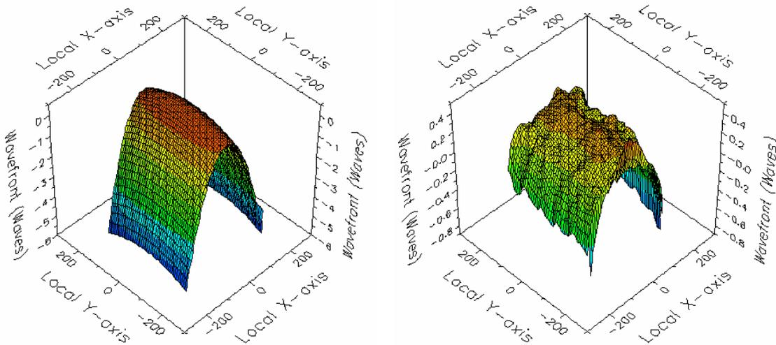
Figure 5 – **The DM corrects better when the power error on the diffraction grating is continuous** – The wavefront of the corrected pulse (right) is narrower and smoother than that of the corrected pulse in Fig. 4. The DM is better equipped to correct for a smooth, continuous error (left).
