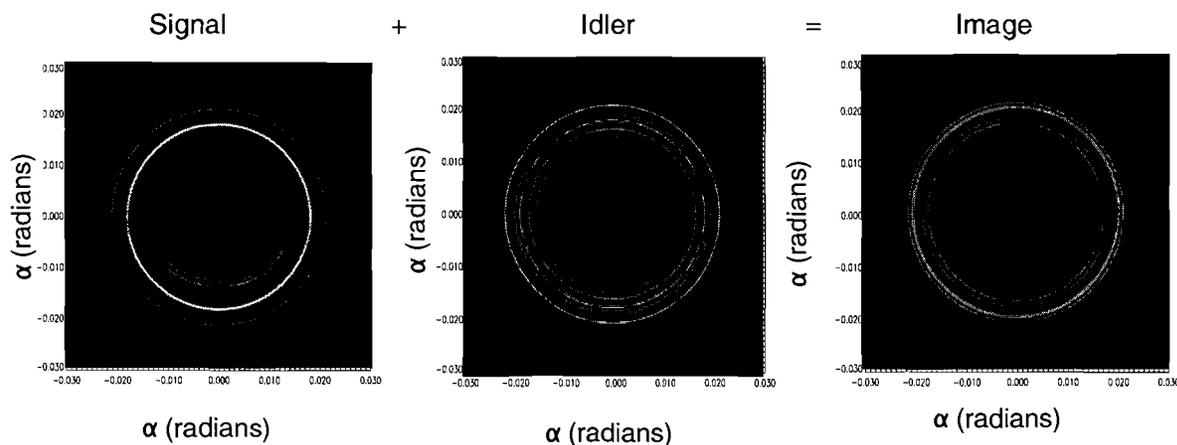
**Figure 6.** These are the images of the signal and idler if taken by a camera at the end of the crystal. Notice the two rings of maximum total intensity which correspond to the two total intensity peaks seen before for this particular crystal tilt ( $13.5^\circ$ ). The actual image seen at the end of the crystal is a combination of the signal and idler and has characteristics of both.
