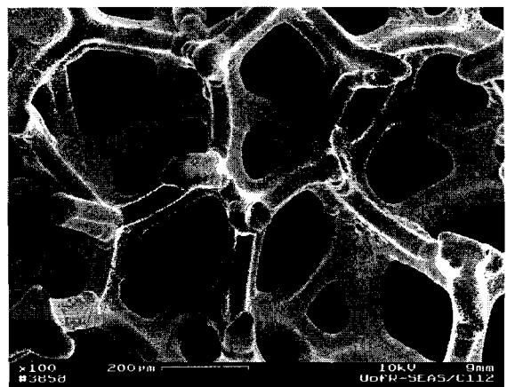
nickel foam. The foam had very large pores with diameters between 450 to 500  $\mu\text{m}$ . The structure of the foam was uniform over the whole surface.
