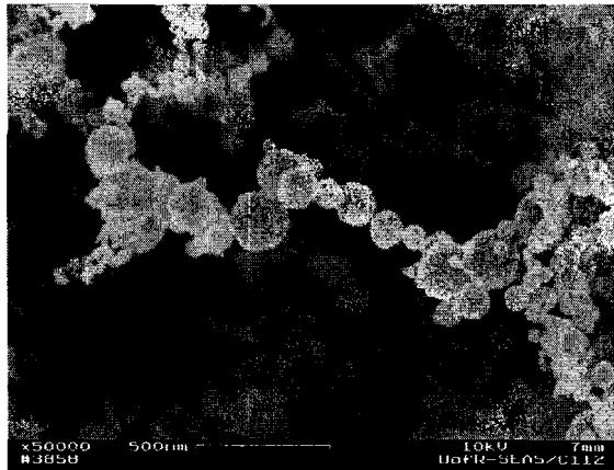
gold was made in house, and intended as a coating for the current Ta foils or alternate metal foams to improve reflectance characteristics. Fluffy gold excelled in the area of reflectance, with only 2.5% of light reflected at 350 nm. SEM scans showed an interesting spherical shape to the deposited fluffy gold. The photo on the left was also
