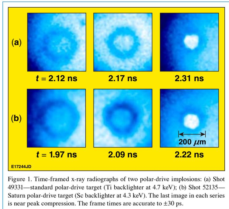
Figure 1. Time-framed x-ray radiographs of two polar-drive implosions: (a) Shot 49331—standard polar-drive target (Ti backlighter at 4.7 keV); (b) Shot 52135—Saturn polar-drive target (Sc backlighter at 4.3 keV). The last image in each series is near peak compression. The frame times are accurate to  $\pm 30$  ps.
