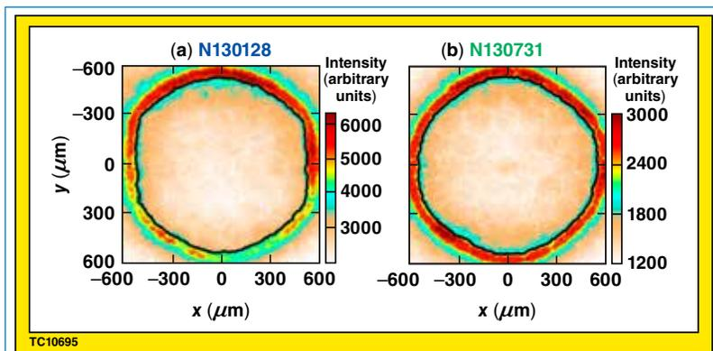
Figure 2. (a) A NIF PD implosion. (b) A NIF PD implosion showing improved sphericity compared to the earlier implosion in (a).
