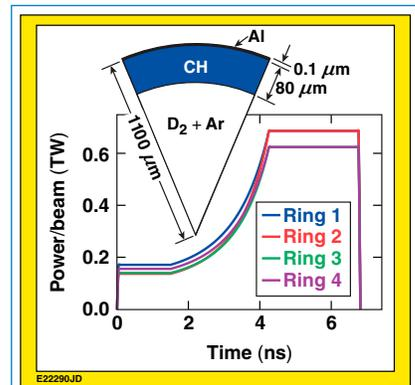
Figure 1. (a) The target used in the National Ignition Facility polar-drive (NIF PD) implosions. (b) The typical laser pulse shapes used in the designs.
