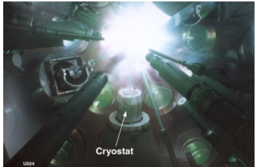
Fig. 1 Cryogenic target positioner used to place a 4-mm pointing sphere at chamber center.
