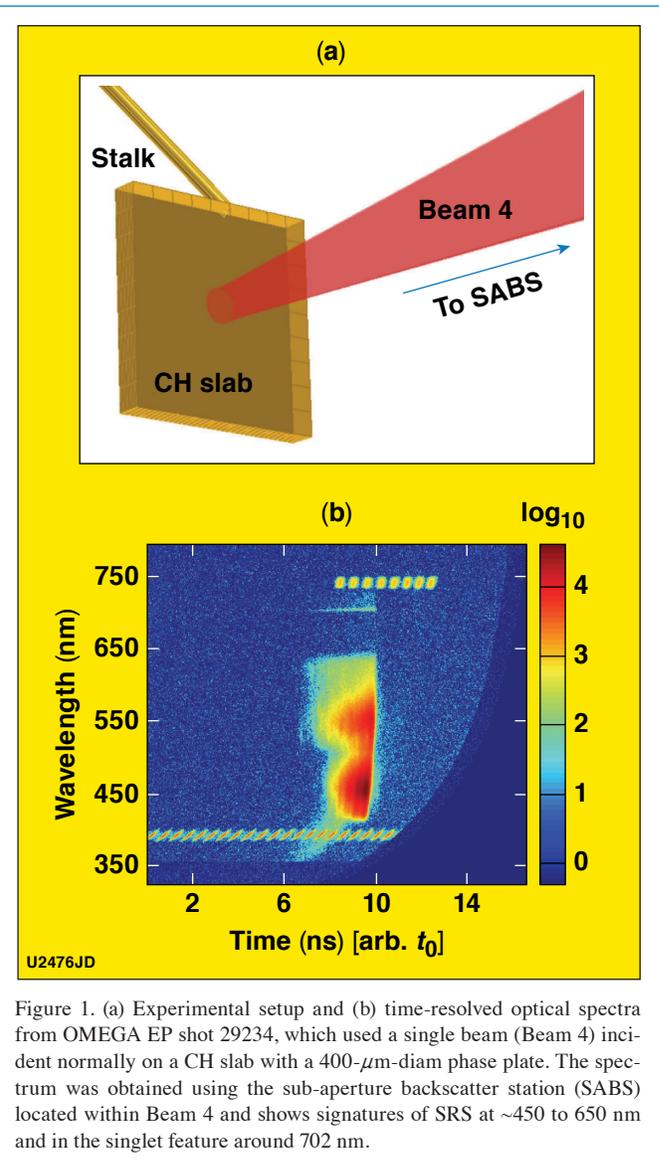
Figure 1. (a) Experimental setup and (b) time-resolved optical spectra from OMEGA EP shot 29234, which used a single beam (Beam 4) incident normally on a CH slab with a 400- $\mu\text{m}$ -diam phase plate. The spectrum was obtained using the sub-aperture backscatter station (SABS) located within Beam 4 and shows signatures of SRS at  $\sim 450$  to 650 nm and in the singlet feature around 702 nm.
