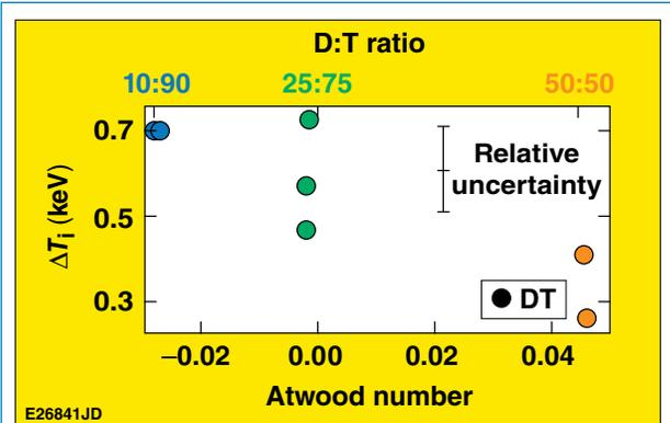
Figure 2. Experimental ion-temperature variation versus fuel D:T ratio and Atwood number.
