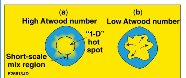
Figure 1. (a) Schematic illustrating the hypothesis that short-scale RT growth in high-Atwood-number implosions prevents fuel from flowing into cold bubbles as happens in (b).
