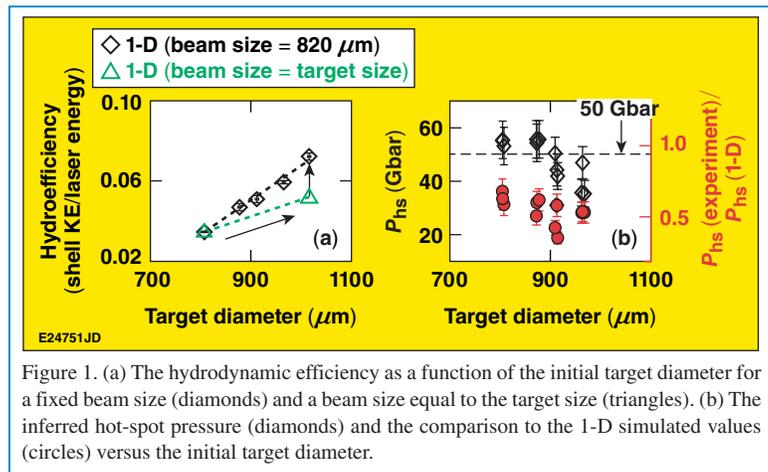
Figure 1. (a) The hydrodynamic efficiency as a function of the initial target diameter for a fixed beam size (diamonds) and a beam size equal to the target size (triangles). (b) The inferred hot-spot pressure (diamonds) and the comparison to the 1-D simulated values (circles) versus the initial target diameter.
