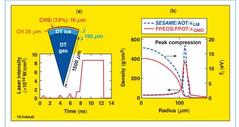
Figure 1. (a) The model-predicted pulse shape for a direct-drive, low-adiabat ( $\alpha \approx 2$ ) ignition design for the National Ignition Facility (NIF), where the insert is the schematic diagram of the NIF target; (b) comparisons between the traditional model prediction (blue curves) and the simulation using the first-principles (FP)–calculated properties of DT (red curves), in which the density and ion temperature are plotted as a function of radius at peak compression.
