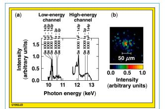
Figure 1. (a) The spatially integrated HSXRS spectrum recorded using a slit is shown with the spectral locations of the Ge K-shell emissions identified. The lower- and higher-energy channels are recorded 300 ps and 200 ps before bang time, respectively. (b) HSXRS image of NIF implosion core in Ge–He<sub> $\alpha$ </sub> emission at 10.2 keV recorded ~100 ps before bang time. The bright spot has a FWHM of ~25  $\mu$ m, which is smaller than the implosion core diameter of ~60  $\mu$ m.
