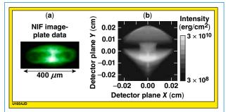
Figure 2. (a) Time-integrated x-ray image of the implosion taken from an image plate. (b) Simulated time-integrated image shows an illuminated oblate imploded shell and a self-emitting prolate core with filtering ( $\sim h\nu > 5.5$  kV) and GXD response.
