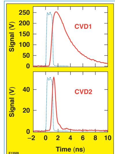
Figure 2. Signals from two CVD detectors (solid red lines) relative to a 1-ns square laser pulse (dotted blue) for shot 37591 (thin shell, DT fill) with  $7.9 \times 10^{13}$  neutron yield.
