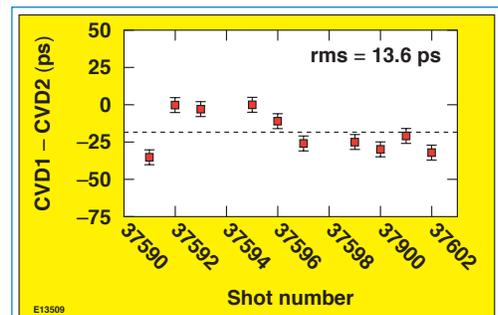
Figure 3. The time difference between the two CVD diamond detectors as a function of shot number.
