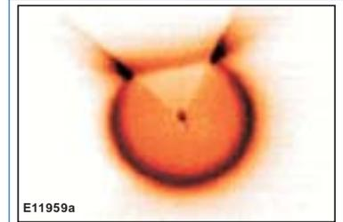
Figure 2. X-ray pinhole camera photograph of a direct-drive cone-in-shell target implosion from the recent OMEGA experiments. Note the opaque area corresponding to the cone inside the shell and the core emission at the center of the shell.
