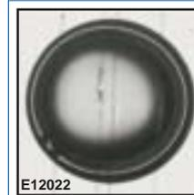
Figure 3. A shadowgraph of the capsule imploded on shot 28969. The asymmetry in the ice thickness is apparent.
