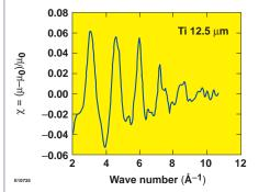
Figure 2. Measured relative modulation of the absorption in Ti derived from Fig. 1 as a function of the wave number of the ejected photoelectron (following *K*-shell photoionization).
