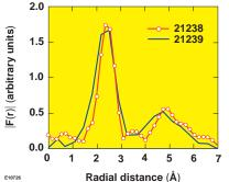
Figure 3. Fourier transform of the spectrum in Fig. 2, yielding the charge distribution around the absorbing Ti atom in the crystal. The spectrum for two consecutive OMEGA shots shows consistency. The weaker peak, due to the second shell of nearest neighbors, is sensitive to order reduction due to shock heating.
