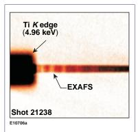
Figure 1. EXAFS modulation observed above the Ti *K* edge, measured by a CID x-ray spectrometer. Ti foil is backlit by an OMEGA-imploded target.
