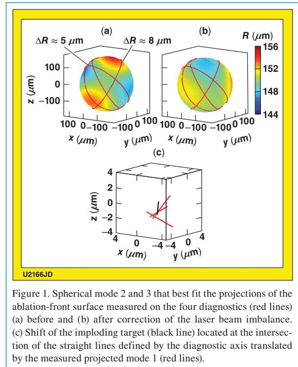
Figure 1. Spherical mode 2 and 3 that best fit the projections of the ablation-front surface measured on the four diagnostics (red lines) (a) before and (b) after correction of the laser beam imbalance. (c) Shift of the imploding target (black line) located at the intersection of the straight lines defined by the diagnostic axis translated by the measured projected mode 1 (red lines).
