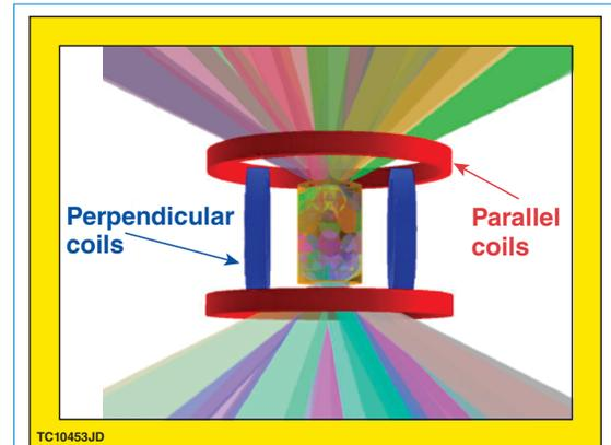
Figure 1: A (VISRAD) model showing the view of the target with both sets of coils present. In practice, only one set is used at a time.
