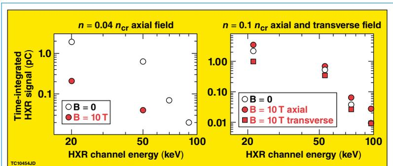
Figure 2: (a) Hard x-ray energy spectra at low density and (b) high density with and without an external magnetic field.
