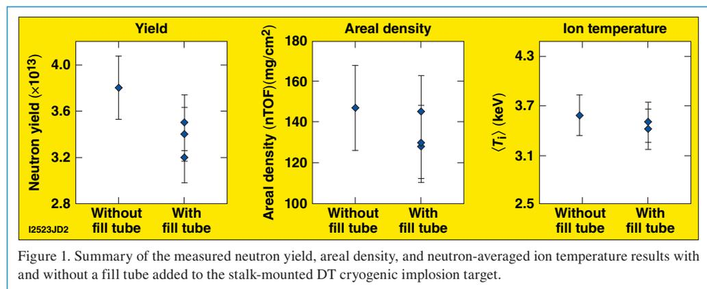
tube, but the difference is within the error bar. These results are encouraging news for the future fill-tube targets on OMEGA. Future experiments will explore the effects of the fill tube on lower-adiabat, higher-convergence DT cryogenic implosions.
